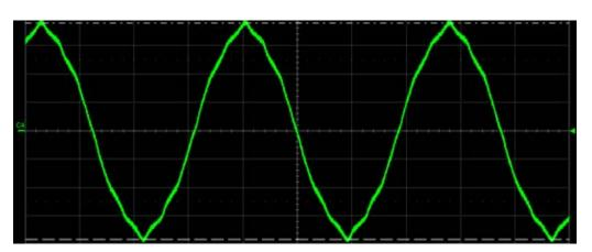
✓ Measured EMF Amplitude = 84.5 V/krpm L-L
