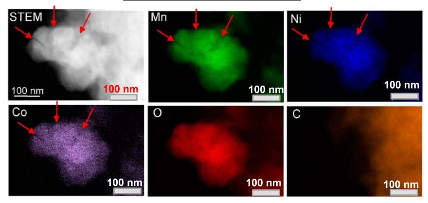
> STEM image and Mn, Ni, Co, O, C, EDS maps showing the crack formation in LNMCO after 60 cycles; the red arrows indicate the crack locations in the image and maps
