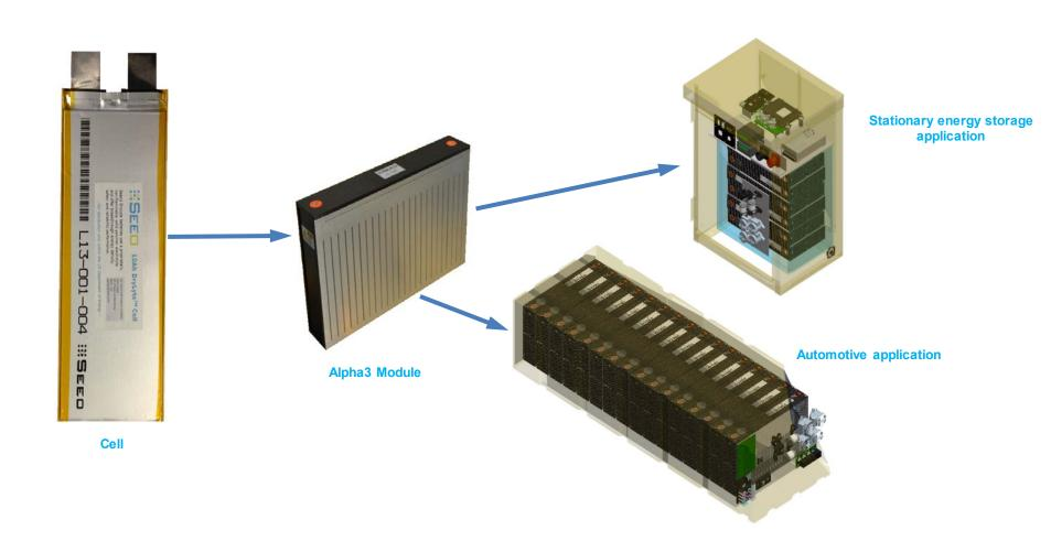
High voltage cells developed w/ support from the VT program will be scaled-up in Seeo's pilot facility & will utilize existing BMS and thermally managed module technologies
