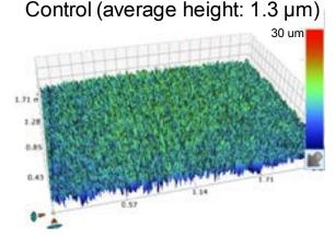
Hydro-Québec and Company B have statistically lower AC interfacial impedance and surface roughness than the Control Lithium
