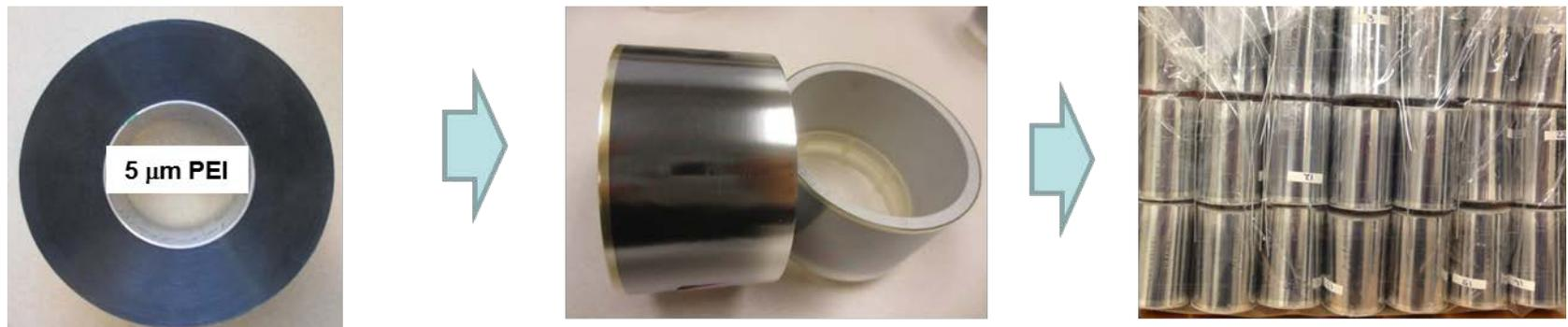
**Disregard the challenges for thinner PEI films at metallization and capacitor winding, capacitors were produced. Yield is to be improved.**
