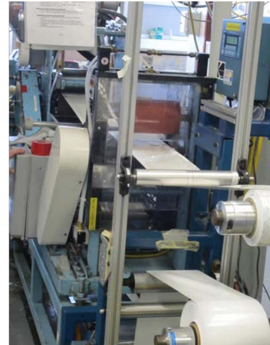
Controlling screw speed, film take-up speed of carrier, die lip gap and temperature, carrier, etc.
