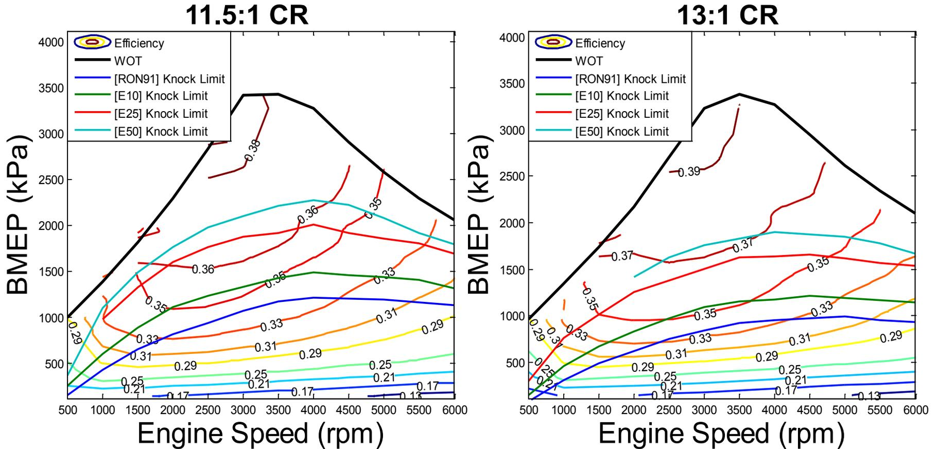
Effects of higher compression ratio and boost on part-load efficiency determined.
