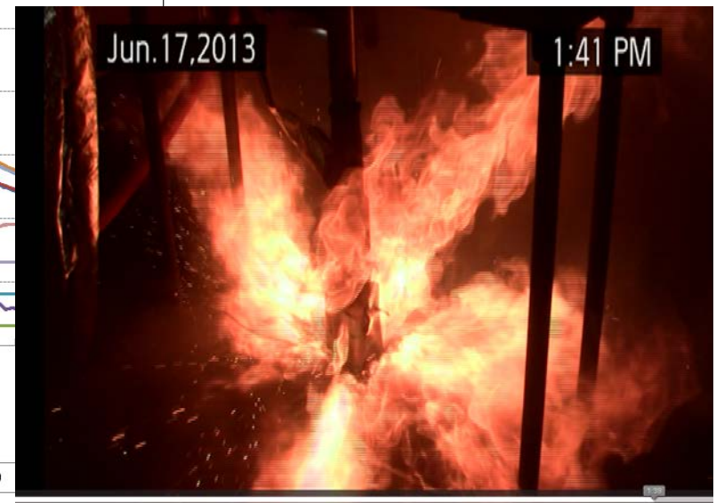
Complete propagation of a single point failure in the 1S10P pack
