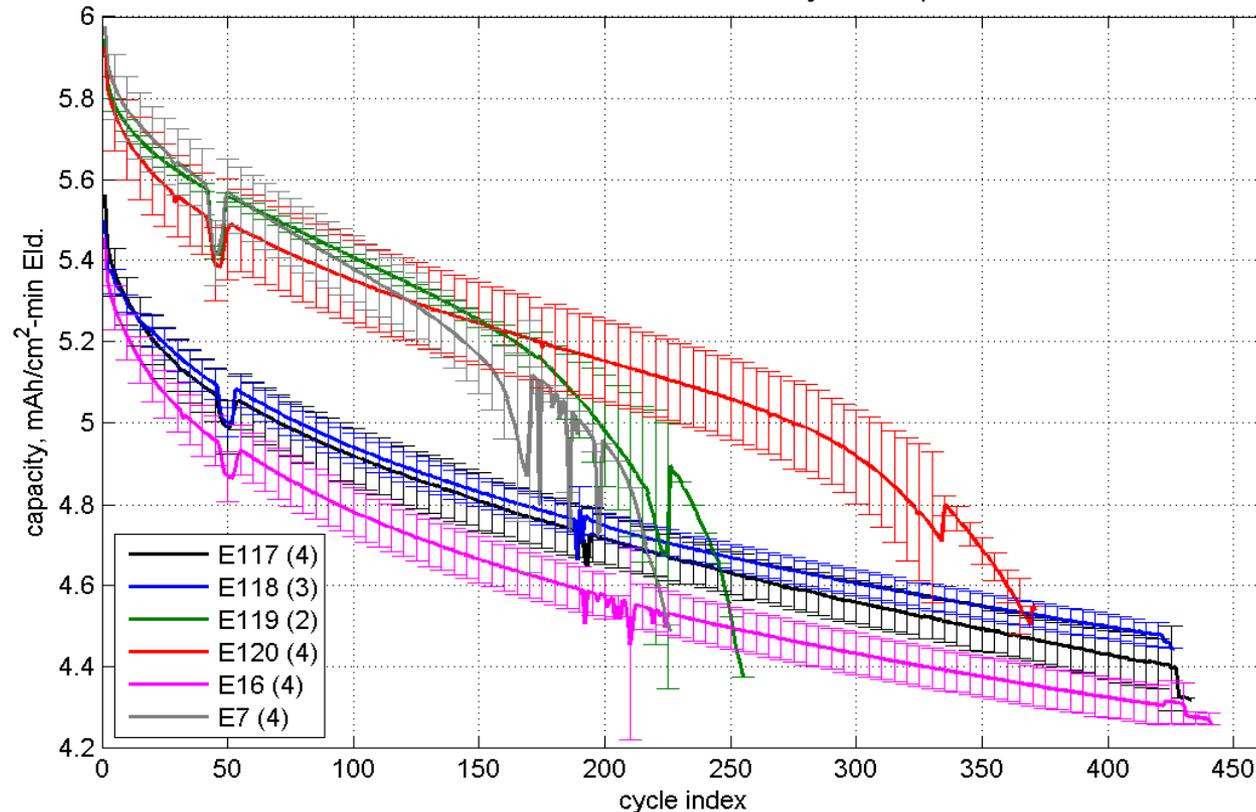
Various electrolyte formulations and additives strongly affect the cycle life in full cells
