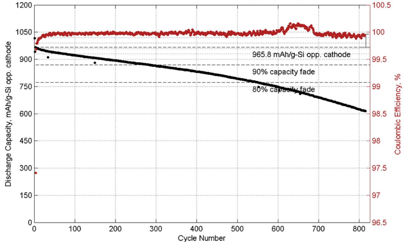
Both Si anode structure and coulombic efficiency are stable to 500+ cycles
