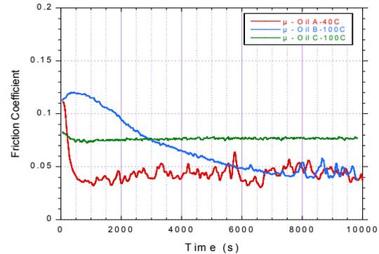
Figure 1: Friction behavior of three different lubricants with different additives
