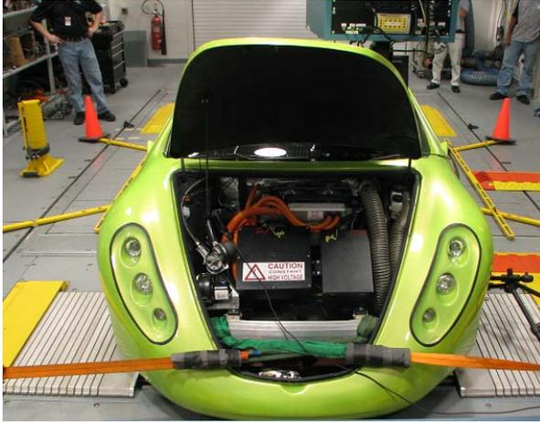
Figure 3. Team Li-Ion (#27) testing on the dynamometer
