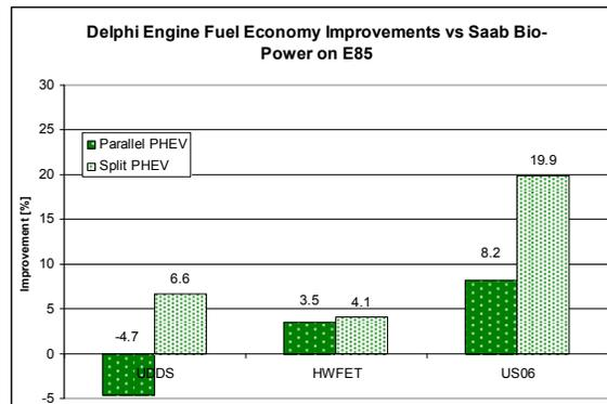
Figure 7 Comparison of Delphi ethanol-optimised PHEV fuel economy results compared to Saab Bio-Power PHEV
