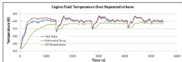
Figure 18. Over-prediction of initial coolant temperature.
