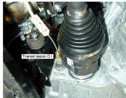
Figure 5. Transmission Oil Temperature Sensor
