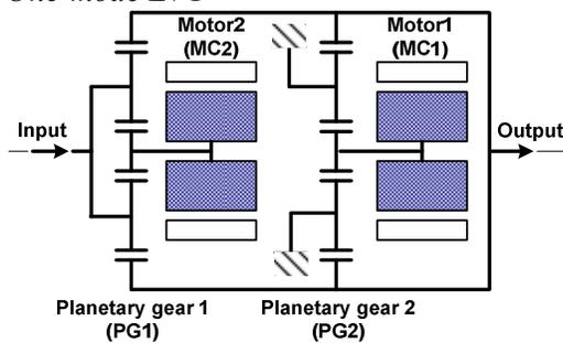
Figure 2. Schematic of the one-mode EVT
