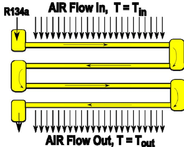
Figure 10. Current Condenser/Evaporator Configuration (Each Layer of Tubes is Represented with one Tube only in this Sketch)
