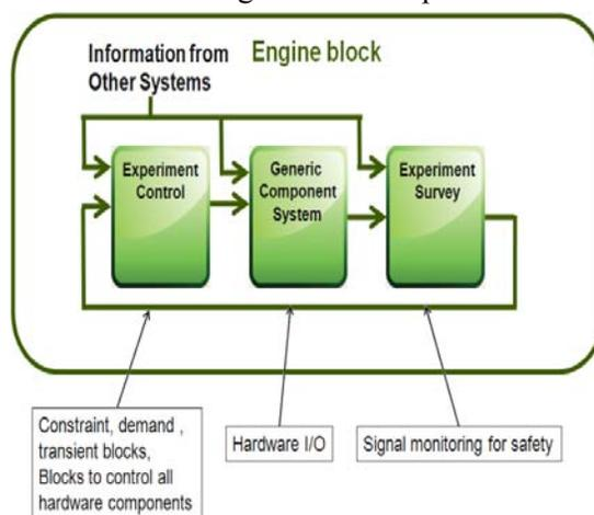
Figure 3. Engine in the loop configuration in Autonomie for easy migration from simulation to engine in the loop testing.
