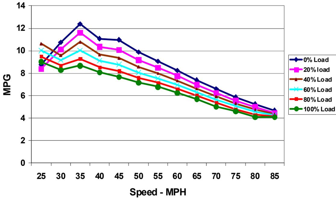
Figure 4: Impact of Vehicle Steady-state Speed on Line Haul Fuel Consumption
