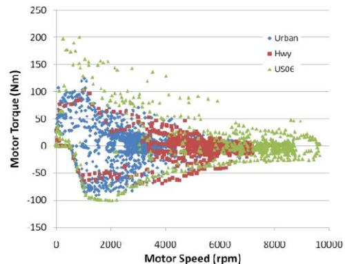
Figure 14. Electric Machine (MG2) Usage
