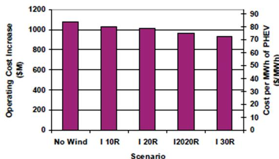
Figure 5: Increased evening loads due to PHEVs reduced the cost of RE generation by about 15%
