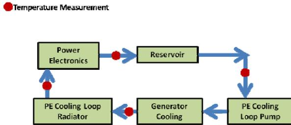
Figure 2. Power Electronics Cooling System and Thermocouple Placement
