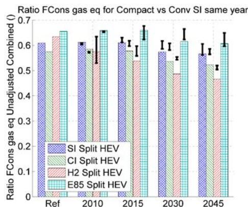
Figure 10. Ratio of Fuel Consumption Gasoline-Equivalent in Comparison to the Conventional Gasoline
