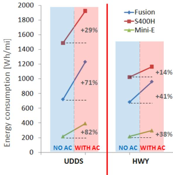
Figure 15: Air-conditioning Impact on Energy Consumption for Different Powertrains
