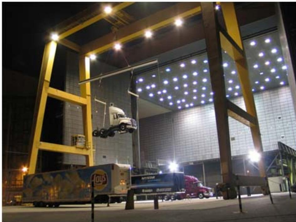
Figure 1. Top) Long-sleeper tractor and 53' straight-frame trailer in the 80'x120' NASA Ames wind tunnel. Bottom) Day-cab tractor being lifted into the wind tunnel test section. The drop-frame trailer, straight-frame trailer, and long-sleeper tractor are visible at the bottom of the photo.
