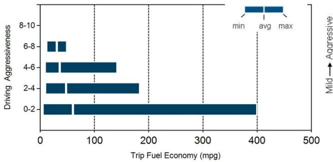
Aggressiveness factor is based on accelerator pedal position. The more time spent during a trip at higher accelerator pedal position, the higher the trip aggressiveness.
