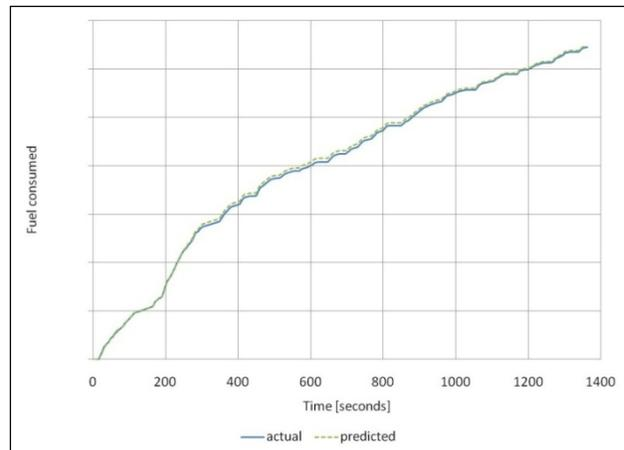
Figure 6. Model-predicted fuel consumed, 266 K UDDS cycle vs. actual recorded fuel consumed. Model < 0.4% predicted integrated value from actual data.
