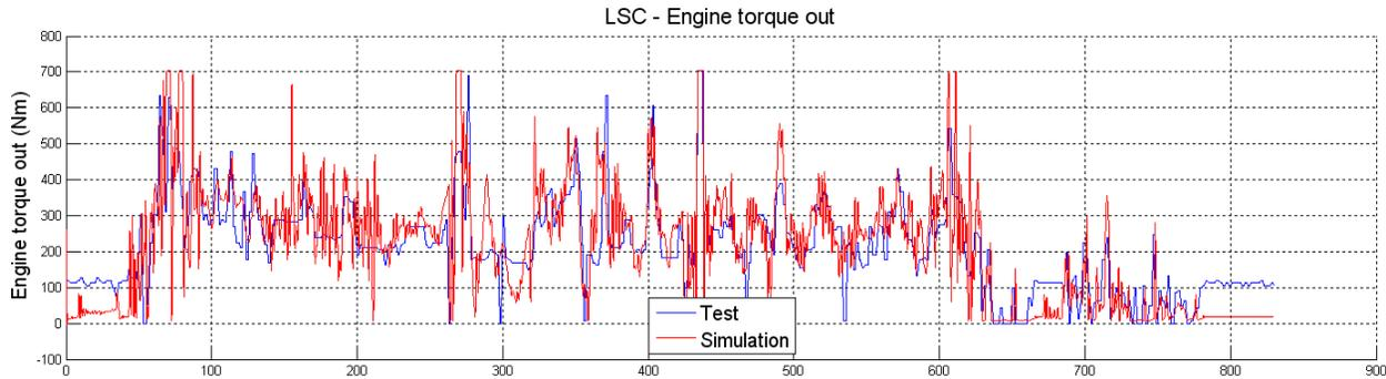
Figure 3: Comparison of Engine Torque on LSC Cycle
