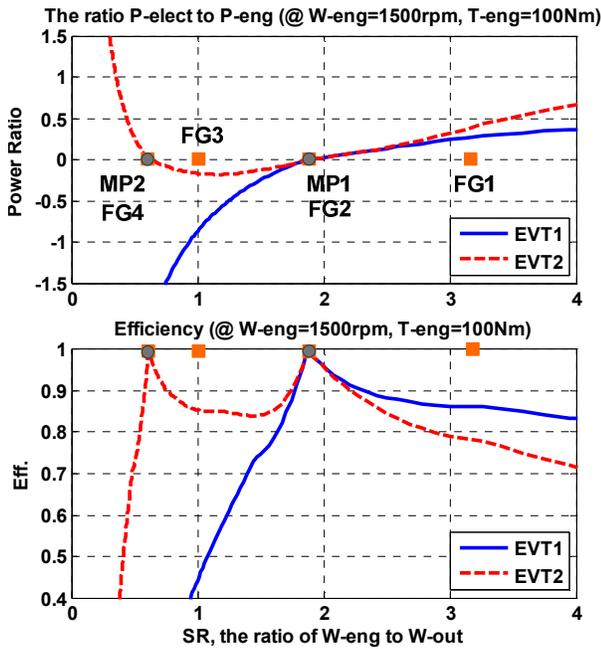
Figure 5. Power characteristics of the two-mode EVT with FGs
