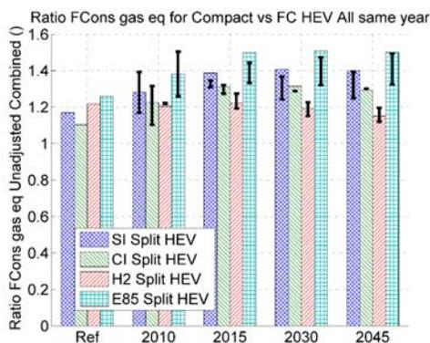
Figure 11. Ratio of Fuel Consumption Compared to the Fuel Cell HEV
