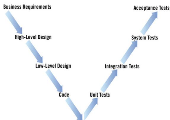
Figure 1: V Diagram for software development
