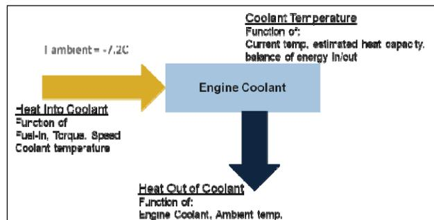
Figure 15. Preliminary coolant model overview.
