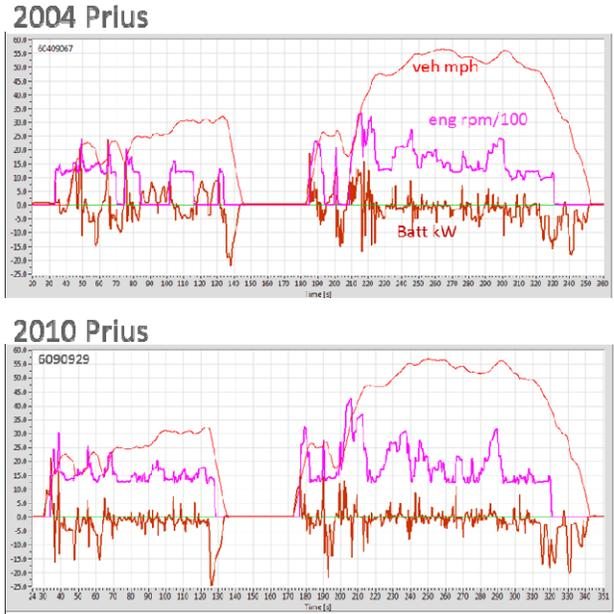
Figure 2. Gen 2 and Gen 3 Prius Comparison of Hot-Start UDDS Data Showing Initial Start Strategy Differences
