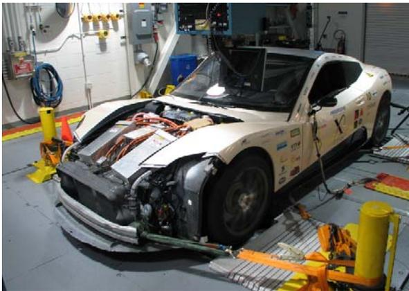
Figure 4. Team RaceAbout (#10) testing on the dynamometer
