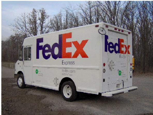
Figure 1. Class 4 P&D Vehicle
