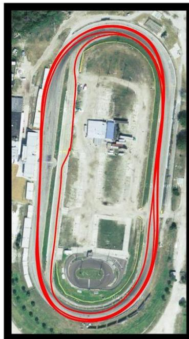
Figure 10. New Smyrna raceway. Red lines indicate the recorded position of the car over five laps. Two warm up laps were allowed that preceded five laps of full effort tracing the same path, followed by one coast-down lap before re-entering the pit lane.
