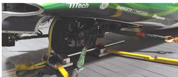
Figure 160. Three-wheel vehicle restraining system
