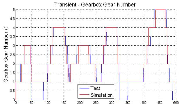
Figure 2: Gear Number Comparison on the Transient Cycle
