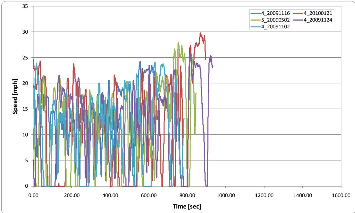
Figure 3. Transit Bus Highway Duty Cycles
