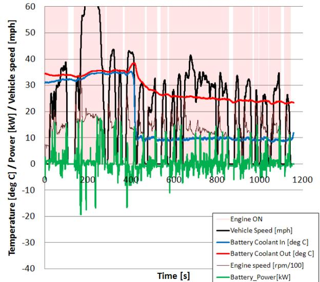
Figure 11: Forced Battery Pack Cooling Using the Air-conditioning System
