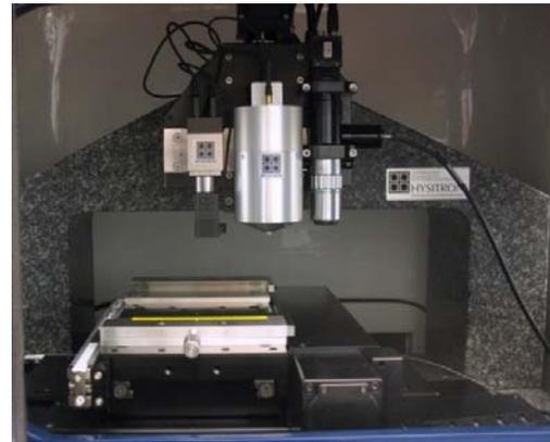
Figure 5: Hysitron instrumented nano mechanical probe system.
