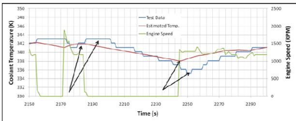
Figure 17. Delay between estimated and actual temperature.
