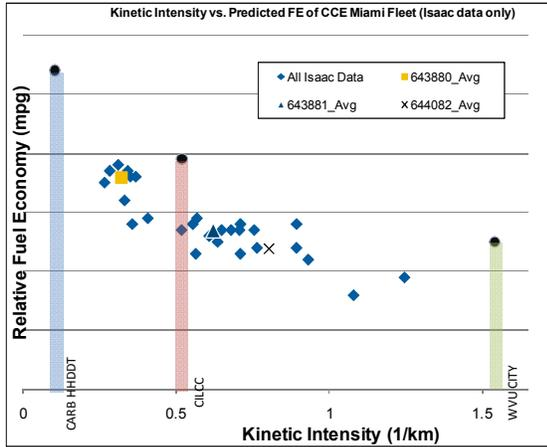
Figure 9. Simulated fuel economy of in-use and standard cycles for CCE vehicles
