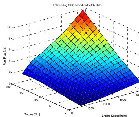
Figure 1. Ethanol-optimised engine fuel flow for PSAT engine model
