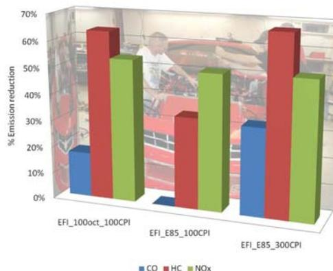
Figure 12. Catalytic converter emissions reduction efficiencies, 100 CPI vs. 300 CPI (E85) vs. E85 (100 CPI) fuel-injected configurations.
