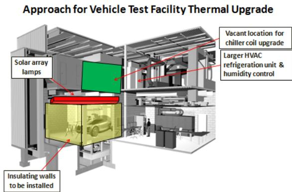
Figure 1. Proposed layout of APRF Upgrade.
