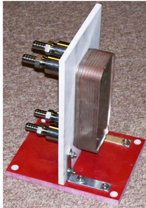
Figure 4. Heat Exchanger (Cooler) Component
