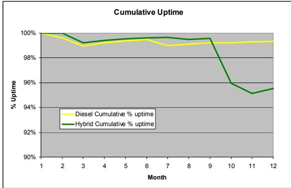
Figure 2. Cumulative uptime of hybrids and diesels
