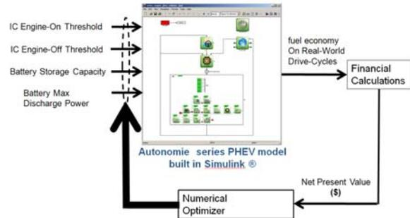
Figure 6. Optimization problem statement: Maximize the NPV by changing battery and control parameters
