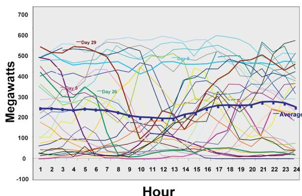
Figure 4. Wind Dynamics are gradual but dramatic while on average the generation is smooth (source: A. Brooks)
