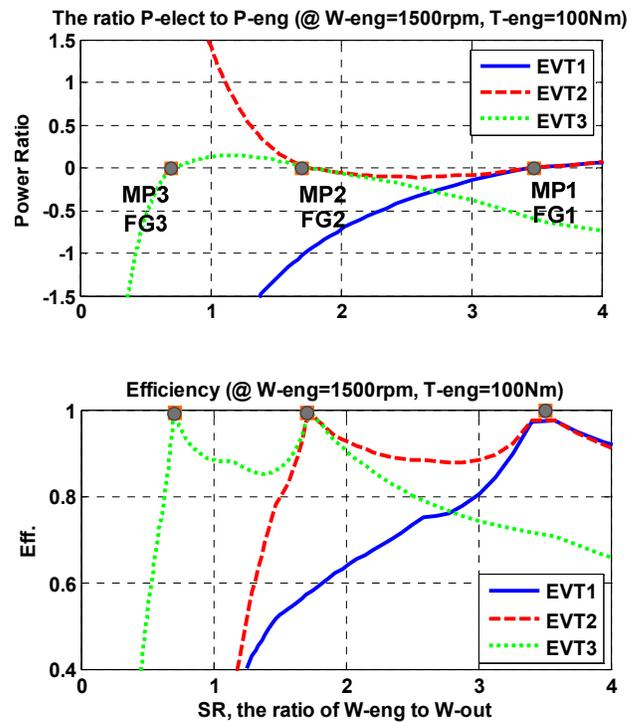
Figure 7. Power characteristics of the three-mode EVT with FGs
