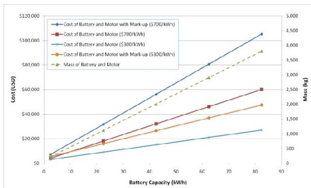
Figure 5. Battery capacity mass and costs
