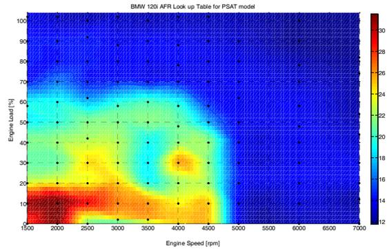
Figure 6. Steady state Air Fuel Ratio as a function of engine speed and load.
