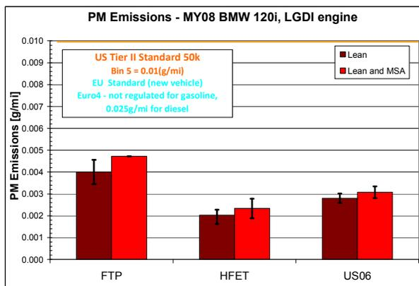
Figure 5. PM emissions as a function of Vehicle Mode and Drive Cycle.
