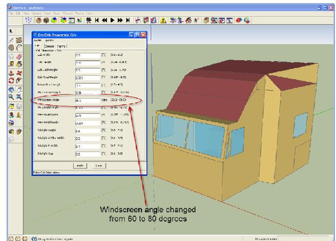
Figure 3. Parametric Cab with Modified Windscreen Angle
