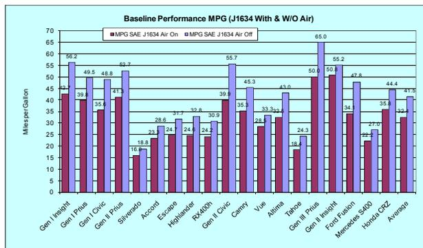
Figure 3. Baseline performance fuel economy test results for SAE J1634 drive cycle testing with the air conditioning on and off.
