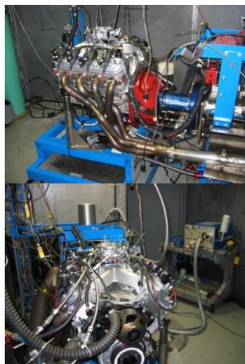
Figure 7. Dynamometer testing configuration for the circle track-525 LS3 engine (top and bottom). MAST Motorsports engine is shown on the right with the SEMTECH DS portable emissions measurement system (PEMS).
