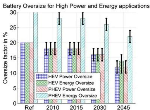
Figure 7. Battery Oversizing
