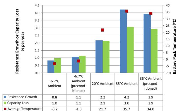
Figure 6. PHEV40s battery degradation rates (left axis) and average temperature (right axis)
