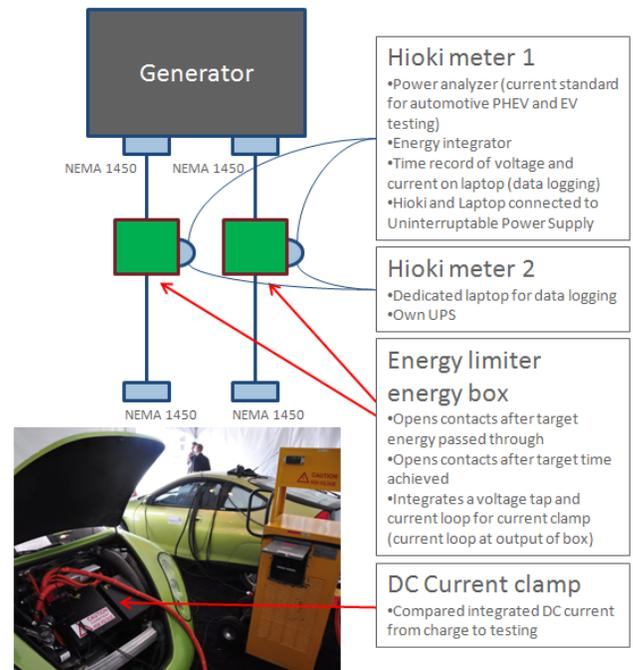
Figure 2. Charge set-up and instrumentation
