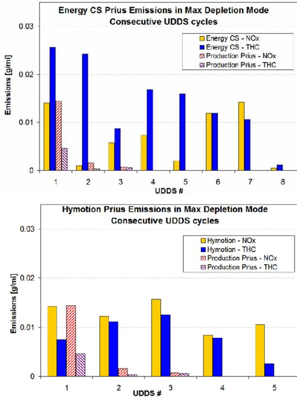
Figure 6. Cycle Emissions Levels for Charge-Depleting Operation Compared to Charge-Sustaining Operation
