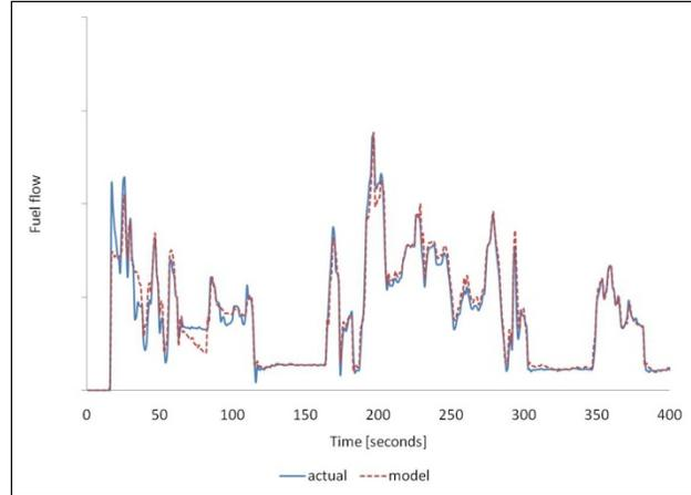
Figure 5. Cold-start model vs. actual fueling detail, initial oil temperature = 20°C, UDDS cycle. Tcoolant = model input for engine temperature.
