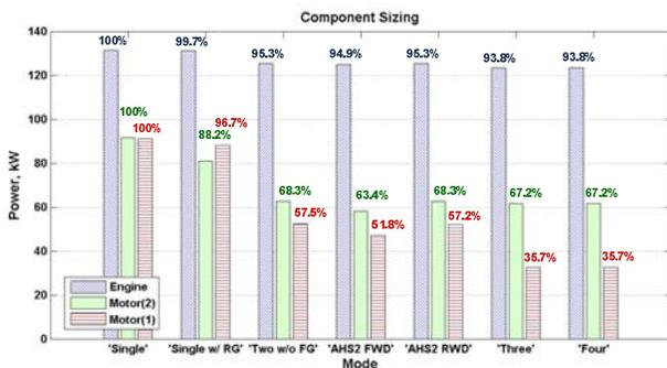
Figure 9. Component sizing results
