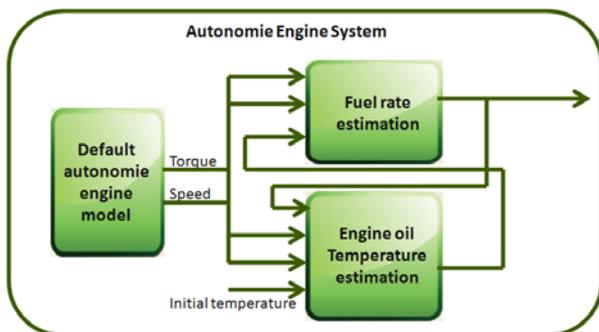
Figure 2. Engine model for efficiency as a function of engine usage, temperature.
