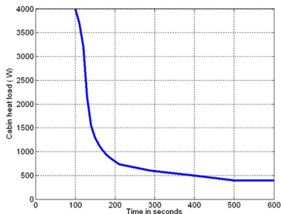
Figure 3. Cabin heating load assumption
