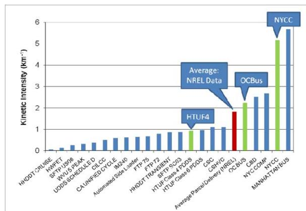
Figure 1: Drive Cycle Kinetic Intensities
