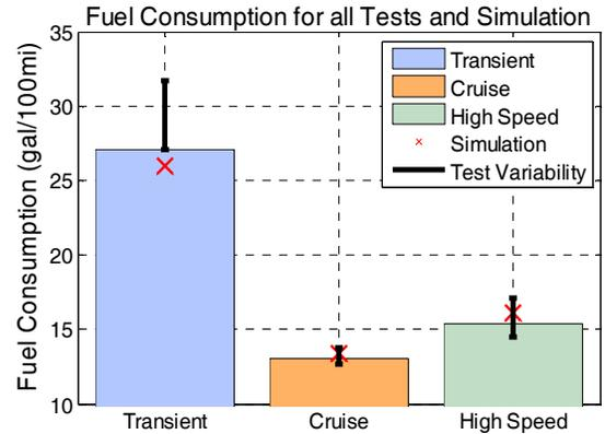
Figure 3. Simulation Results within Test-to-test Uncertainty
