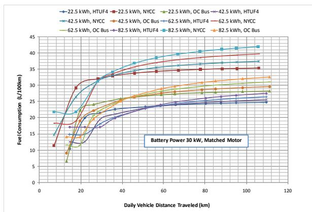
Figure 3: Fuel consumption by daily distance traveled (30 kW)
