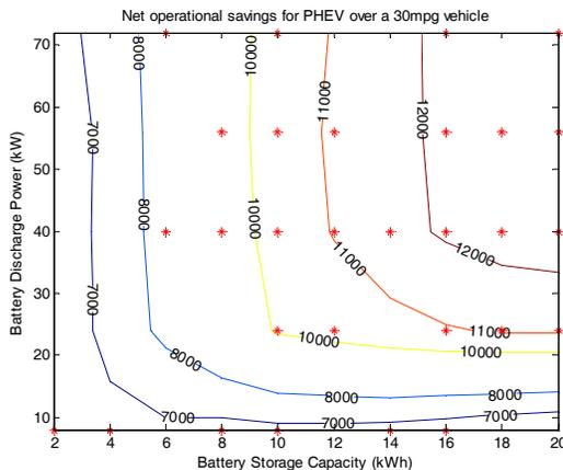
Figure 8. Variation of savings in operational cost with battery size (battery cost not included)
