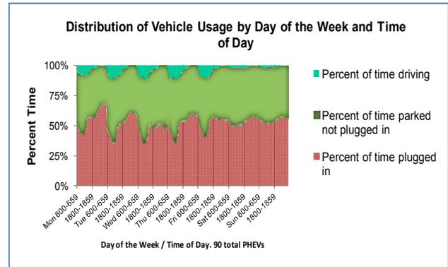
Figure 12. Percent of time 90 Hymotion Prius PHEVs are plugged in, driven, and parked but not plugged in during a one month period.
