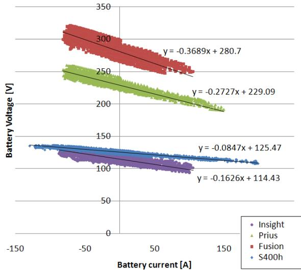
Figure 12: Different Battery Polarization Curve Comparisons
