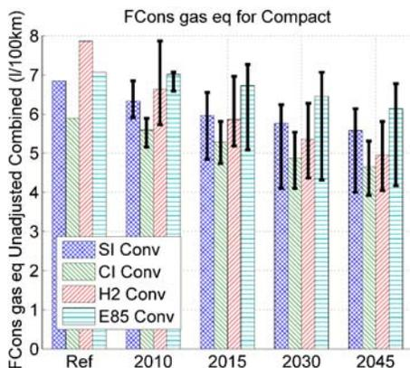
Figure 9. Gasoline-Equivalent Fuel Consumption (unadjusted for conventional midsize cars)
