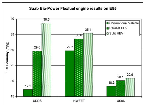
Figure 2. Comparison of Bio-Power HEV fuel economy results compared to conventional vehicle
