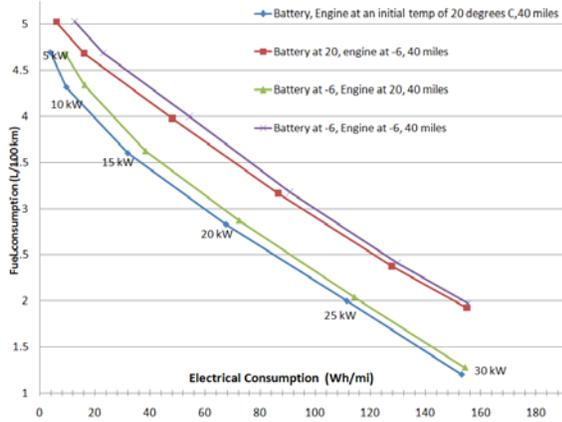
Figure 5. Impact of low temperature of battery and engine (individually and together) on fuel and battery energy consumption for a given distance, different control parameters.
