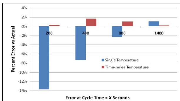
Figure 12. Chart showing amount of error relative to total grams of fuel used for both the single temperature- and time-series temperature-based evaluations at various time segments of the first UDDS cycle.
