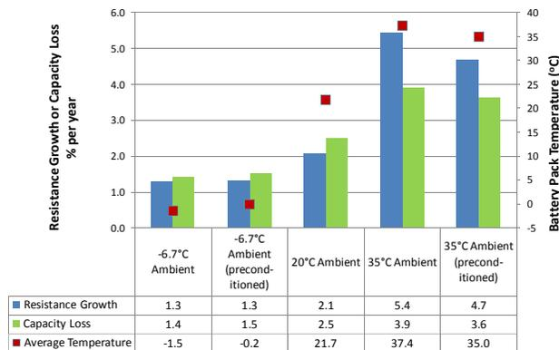
Figure 7. EV battery degradation rates (left axis) and average temperature (right axis)
