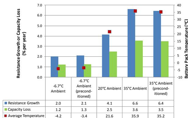
Figure 5. PHEV15 battery degradation rates (left axis) and average temperature (right axis)
