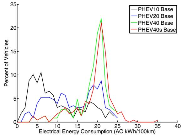
Figure 6. Electrical energy consumption (AC kWh/100km) distribution in Austin data set
