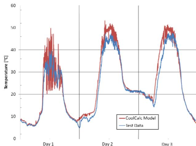
Figure 22. Comparison of Windshield Exterior
