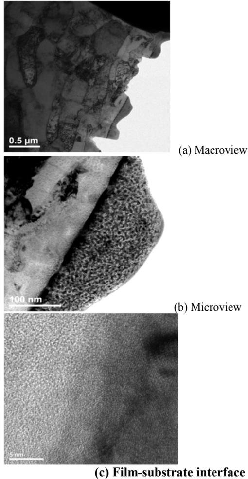
Figure 2: a Tribochemical film from Lubricant A is amorphous.
