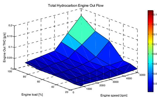
Figure 2. Total hydrocarbon engine out emissions on LAF engine
