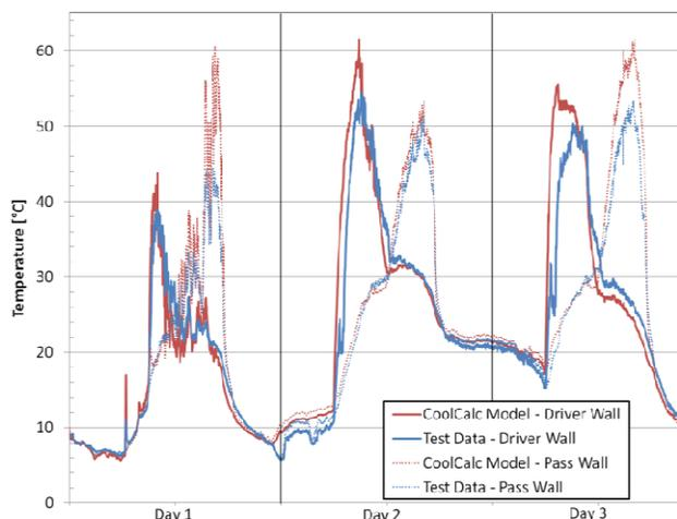
Figure 20. Sleeper Driver and Passenger Exterior Side Walls
