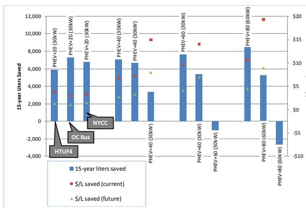
Figure 13. Lifetime liquid fuel displacement and cost effectiveness, 80 km/day
