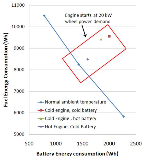
Figure 4. Impact of low temperature of battery and engine (individually and together) on fuel and battery energy consumption for a given distance, and control parameters.
