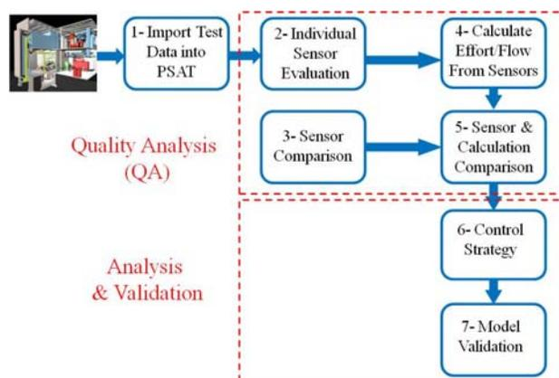
Figure 1. Test Data Analysis Process
