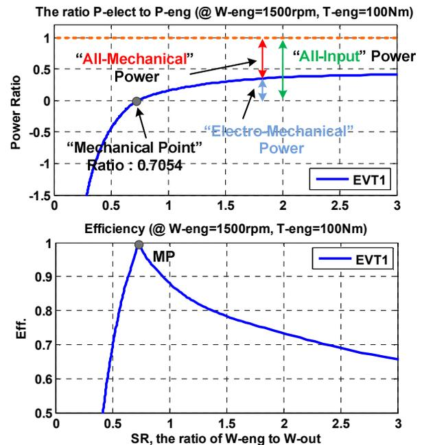
Figure 3. Power characteristics of the one-mode EVT
