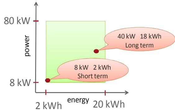
Figure 9. Battery sizes chosen for maximum NPV
