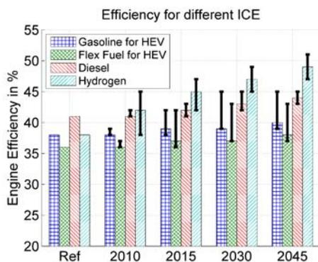
Figure 4. Engine Efficiency Evolution
