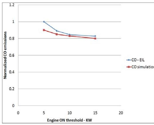
Figure 5: Comparison of CO trends for simulation and EIL.
