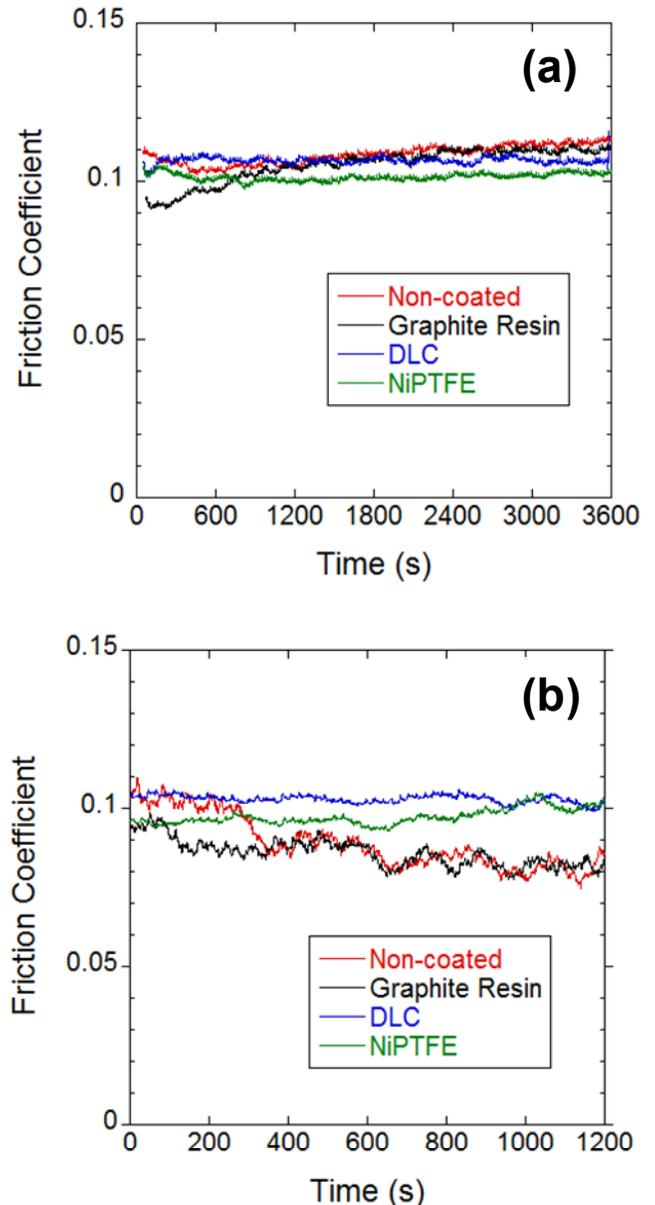
Figure 7: Friction coefficient as a function time for all samples tested using a load of 250 N in (a) fully formulated 10W30 oil at 120°C for 1 hour and (b) PAO10 oil at 20°C for 20 minutes.
