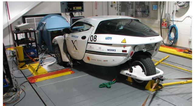
Figure 8. Team ZAP (#08) testing on the dynamometer
