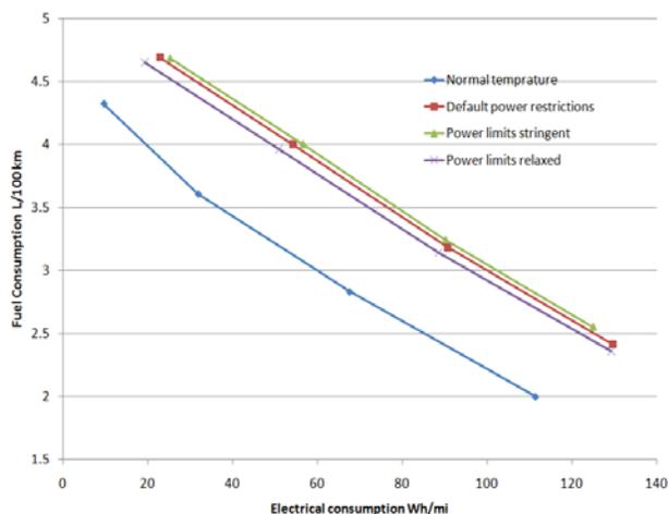
Figure 9: Impact of change in battery power restrictions at cold temperature for 40 miles, LA92.
