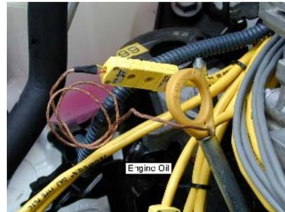
Figure 4. Engine Oil Temperature Sensor
