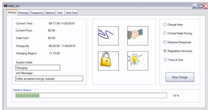
Figure 19. HMI for Controlling the Charging Process
