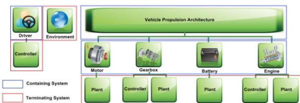
Figure 3: Class diagram of container and terminating systems
