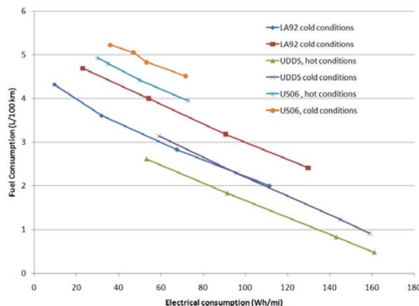
Figure 7. Impact of cold temperature on fuel and electrical consumption for mild and aggressive driving.
