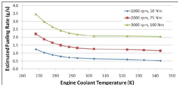
Figure 10. Estimated fuel rate for several representative engine operating points at a range of temperatures.
