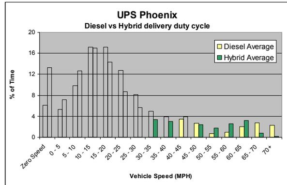
Figure 1. Hybrid and diesel drive cycle statistics
