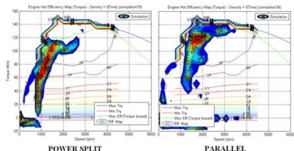
Figure 6 Ethanol-Optimised engine speed histograms in HEV powertrain vehicle engine (UDDS cycle)
