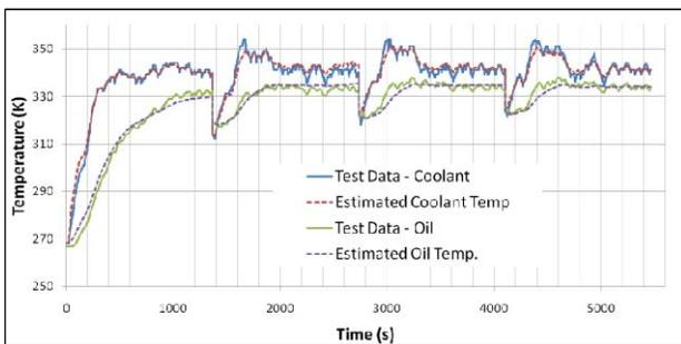
Figure 20. Estimated oil and coolant model vs. actual data.
