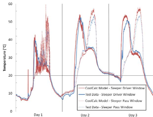
Figure 21. Comparison of Sleeper Interior Side Windows
