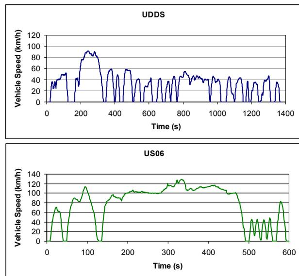
Figure 2. Speed vs. Time Trace for the UDDS and US06 Drive Cycles.
