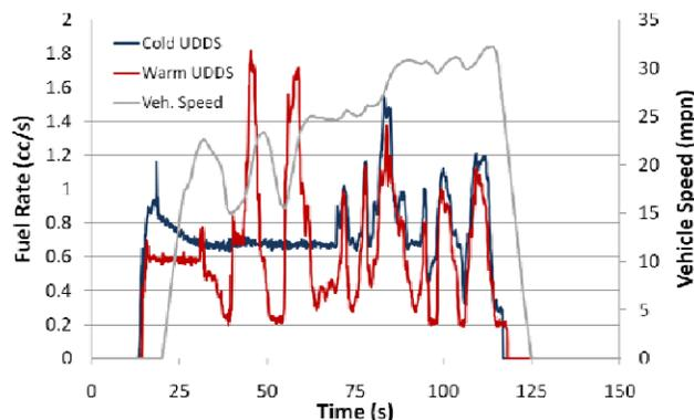
Figure 11. Cold versus Warm Engine Fueling at Engine Start
