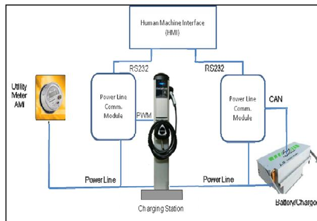
Figure 1: Laboratory test bench setup
