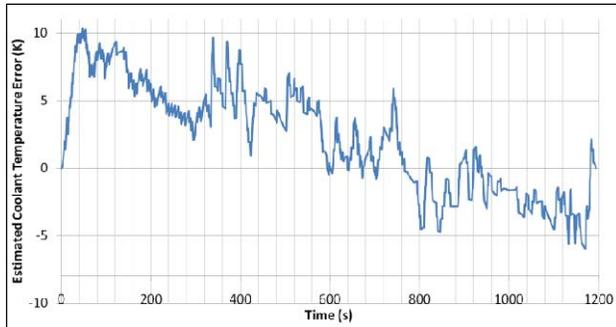
Figure 23. Error of the US06 cycle coolant fit relative to the experimental data.
