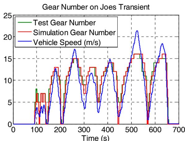
Figure 1. Gear number comparison between test and simulation
