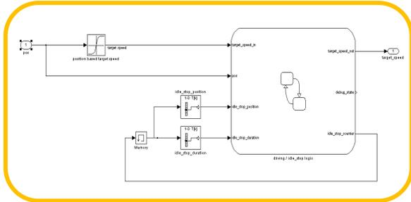
Figure 1. Distance Based Driver Model
