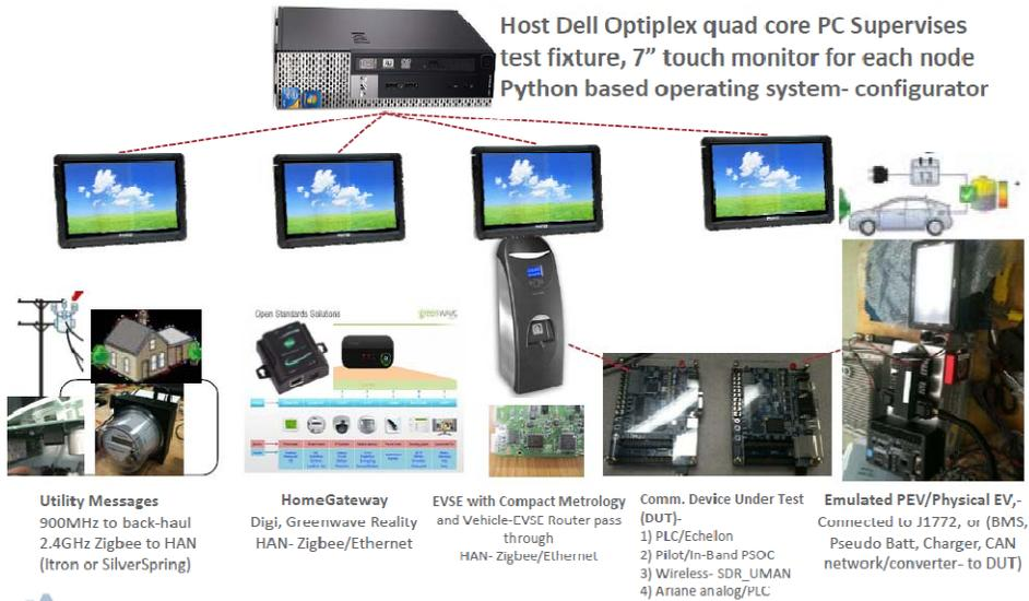
Figure 1 Vehicle-Grid compatibility evaluation test fixture
