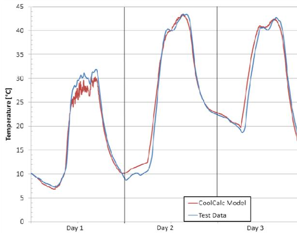
Figure 17. Cab Average Air Temperature Comparison
