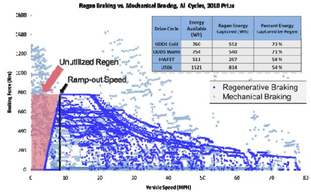
Figure 13. Estimated Regenerative Braking Envelope
