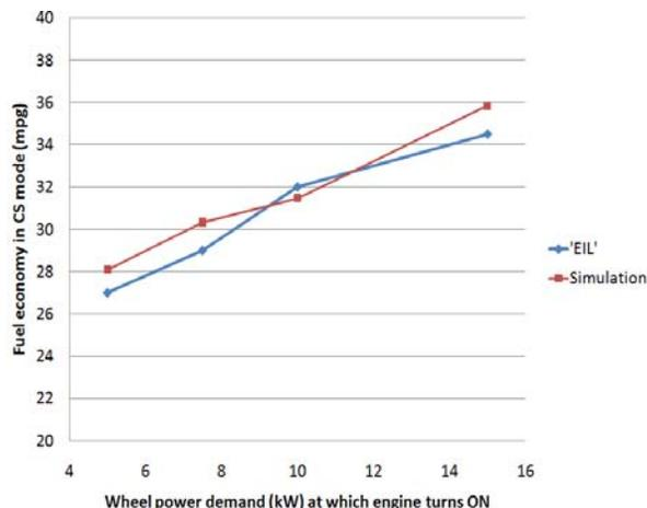
Figure 4: Comparison of the simulation and EIL fuel economy for CS mode of operation.
