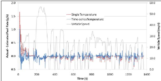
Figure 13. Plot illustrates the error of the predicted fuel rate using the single and time-series temperature estimates over the UDDS cycle.
