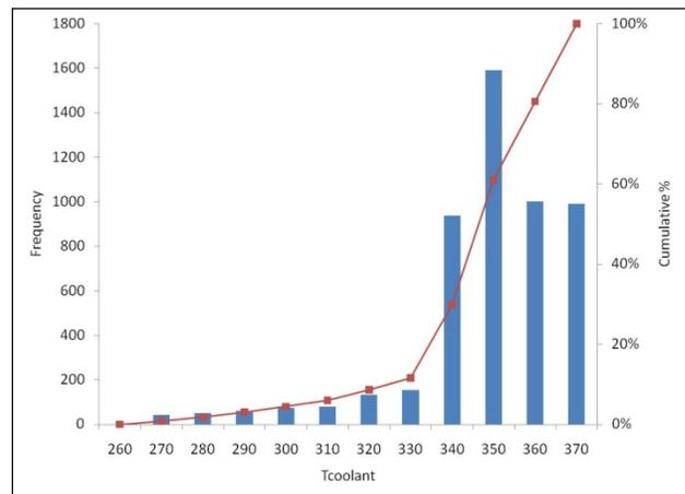
Figure 9. Engine coolant temperature (Tcoolant) histogram, UDDS cycle, 266 K cold start.
