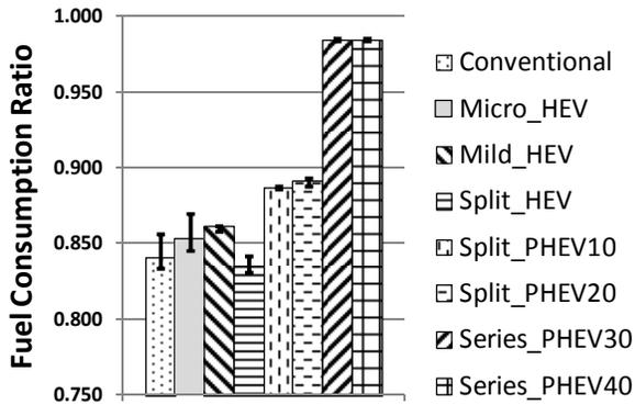
Figure 1. Fuel Consumption Ratios for HCCI vs. Regular Engine with Standard Control Strategy.
