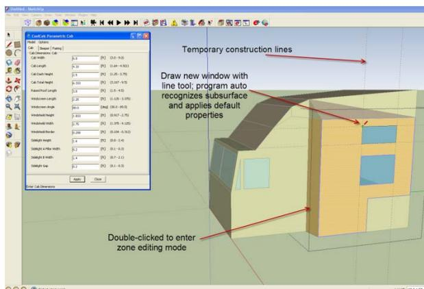
Figure 4. Manual Modification of Geometry - Adding a Sidelight
