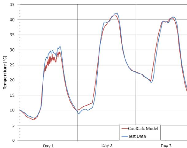
Figure 18. Sleeper Average Air Temperature Comparison
