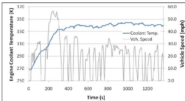
Figure 11. Plot of the engine coolant temperature over the UDDS cycle.
