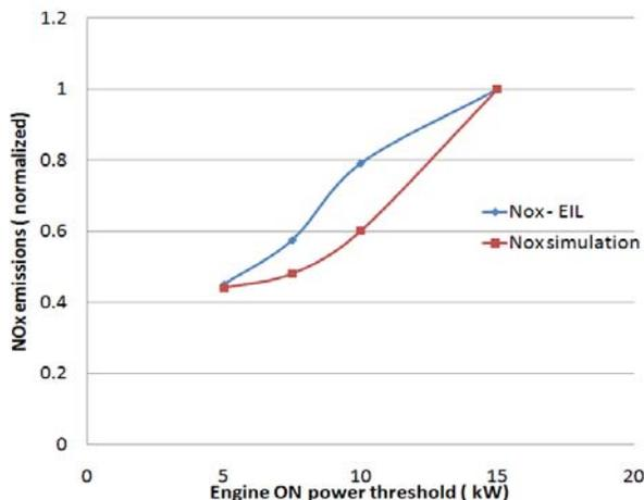
Figure 6: Comparison of NOx trends for simulation and EIL.
