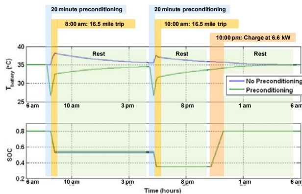
Figure 1. Battery temperature and SOC profiles for PHEV40s, 35°C ambient temperature, with and without thermal preconditioning
