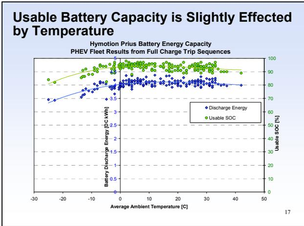
Figure 8. Usable battery capacity by temperature.
