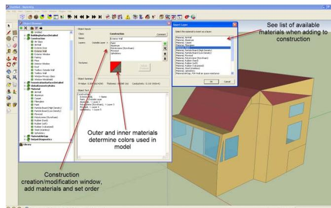
Figure 6. Construction Definition Window
