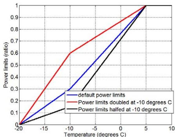
Figure 8: Battery power limit variation at cold temperature.
