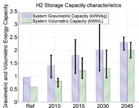
Figure 5. Hydrogen Storage Capacity in Terms of Quantity
