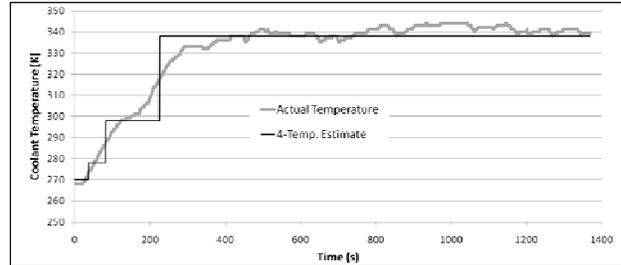
Figure 14. Plot shows the optimal four-coolant temperature options relative to the actual coolant temperature trace.
