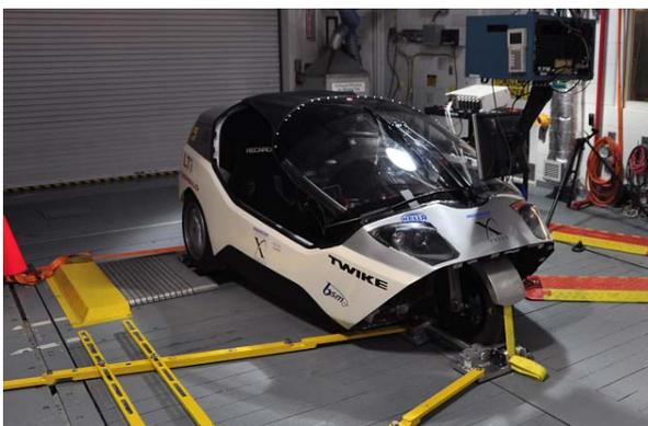
Figure 5. Team TW4XP (#33) testing on the dynamometer
