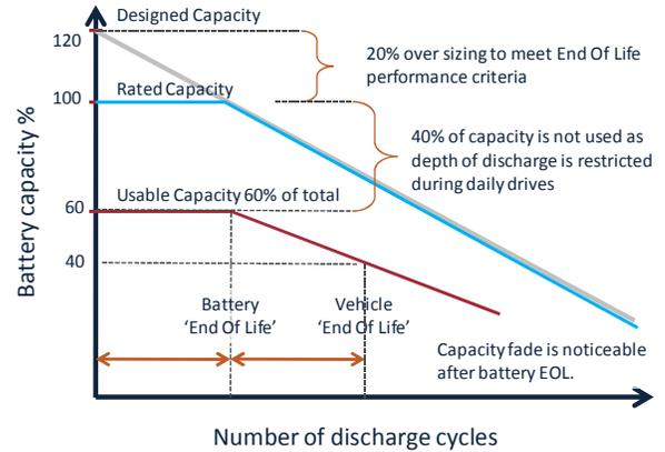
Figure 4. Battery capacity variation with battery use
