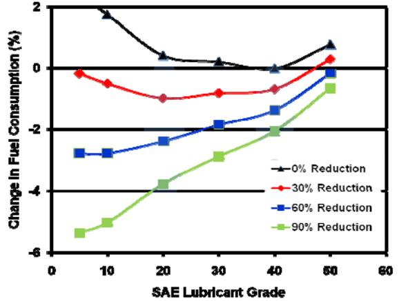
Figure 2: Predicted change in fuel economy as a function of engine lubricant viscosity and boundary friction for an off-road driving schedule (70% idle, mode 2 and 3).
