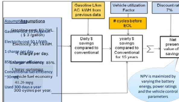
Figure 5. NPV calculation for gasoline savings over vehicle life
