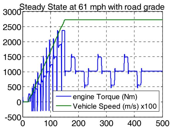
Figure 3. Engine torque during steady state testing
