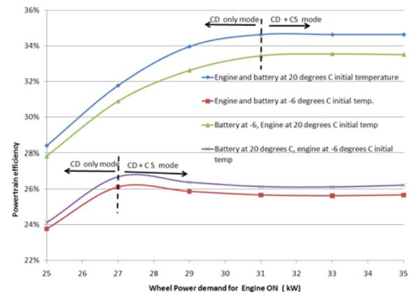
Figure 6. Powertrain efficiency over different engine turn-ON thresholds, with cold initial temperatures for the battery and or the engine.
