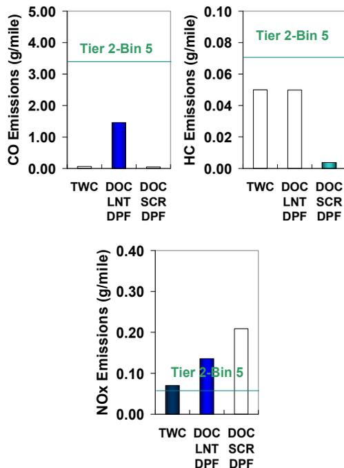
Figure 2. Comparison of cumulative tailpipe emissions from a conventional gasoline-powered passenger HEV with TWC and a diesel-powered HEV with different lean aftertreatment combinations. Simulations are for 80 consecutive UDDS cycles beginning with a cold start.
