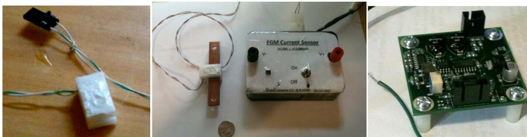
Figure 27 Flux-gate-magnetometer-based current sensor and signal conditioner
