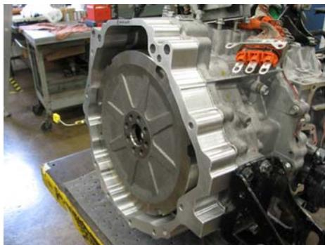
Figure 9. Torque Sensor Spacer
