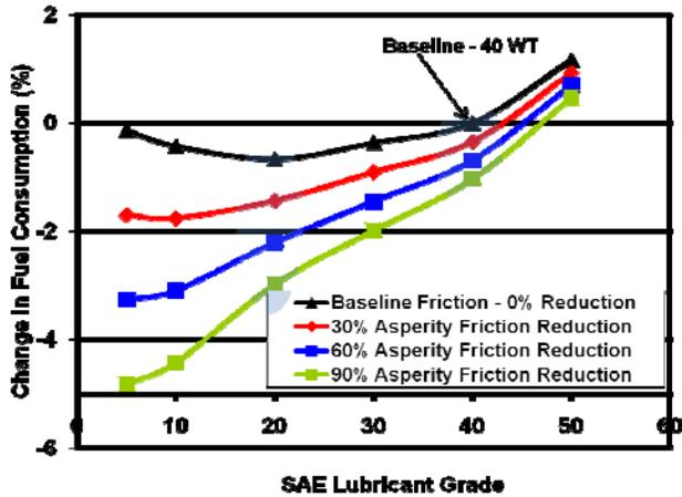
Figure 1.: Predicted change in fuel economy as a function of engine lubricant viscosity and boundary friction for an on-road driving schedule (federal test procedure).
