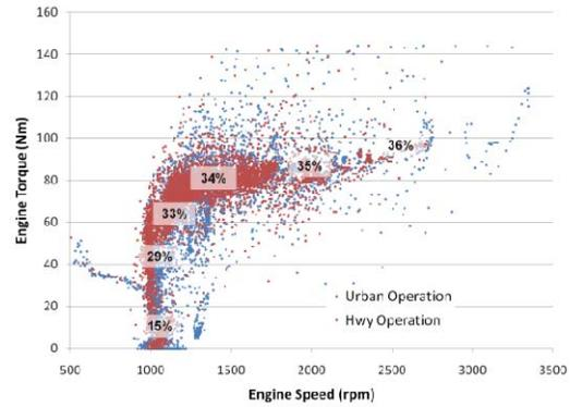
Figure 16. Urban and Highway Engine Usage and Efficiency
