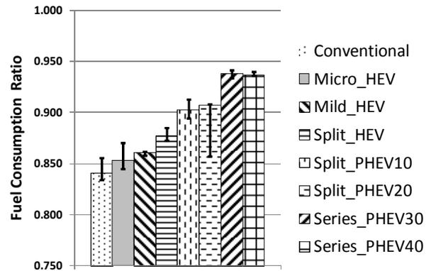
Figure 2. Fuel Consumption Ratios for HCCI vs. Regular Engine (Atkinson for hybrids) with Tuned Control Strategy
