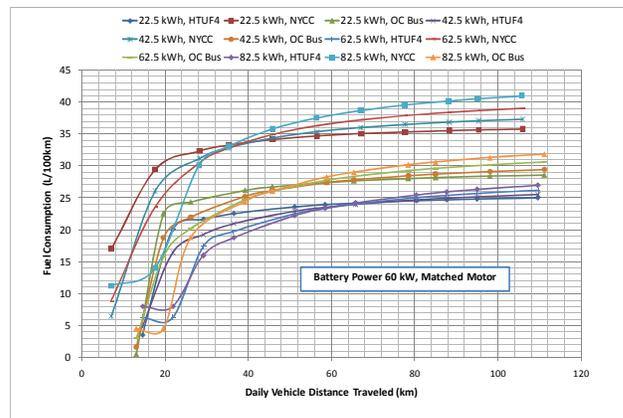
Figure 4: Fuel consumption by daily distance traveled (60 kW)
