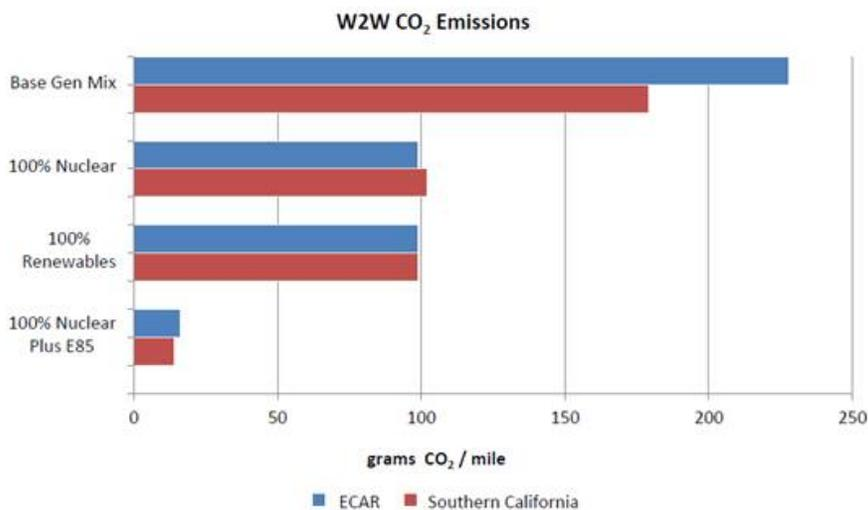
Figure 47: Effects of alternative generation mixes on CO<sub>2</sub> emissions
