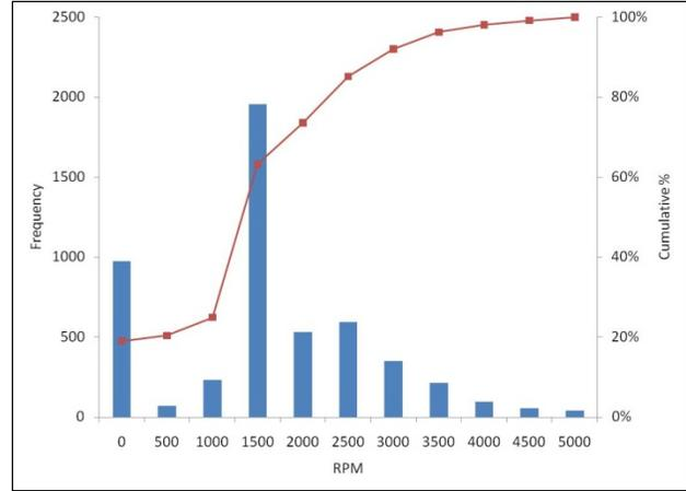
Figure 7. RPM histogram, UDDS cycle, 266 K cold start.
