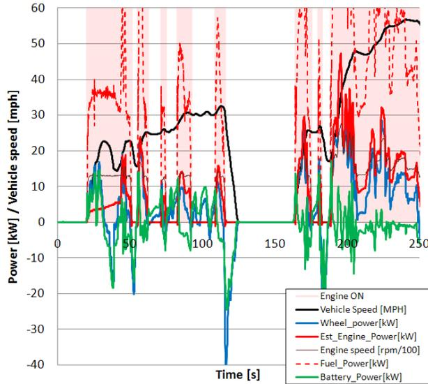
Figure 8. Fusion Operation on a Hot-start UDSS
