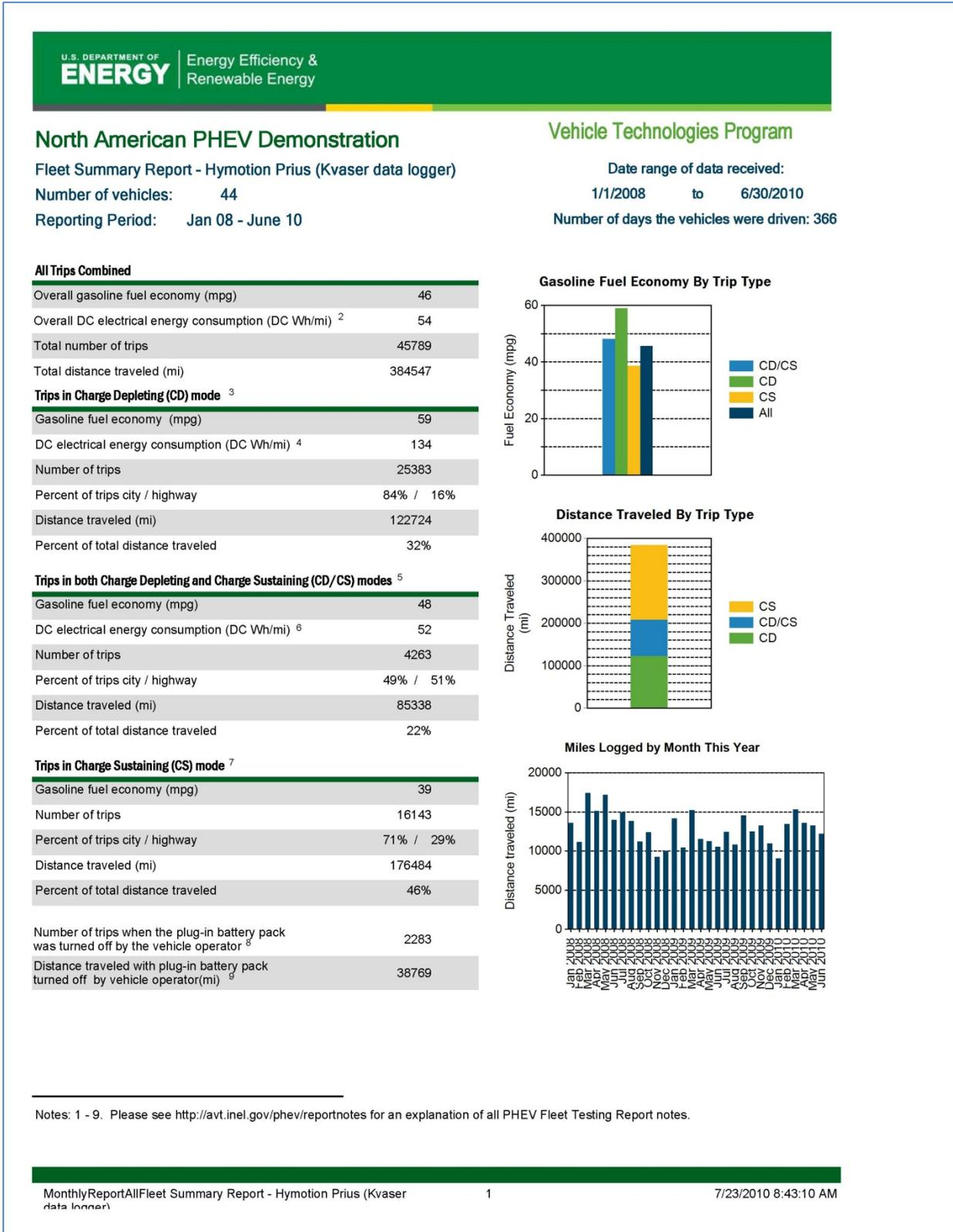
Figure 2. Page 1 of 3 for the PHEV summary report for 44 PHEVs operating January 2008 – June 2010 with onboard Kvaser data loggers.
