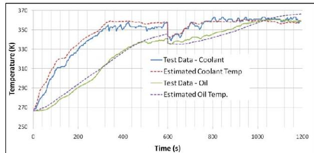
Figure 22. Estimated temperature for repeated US06 cycles.
