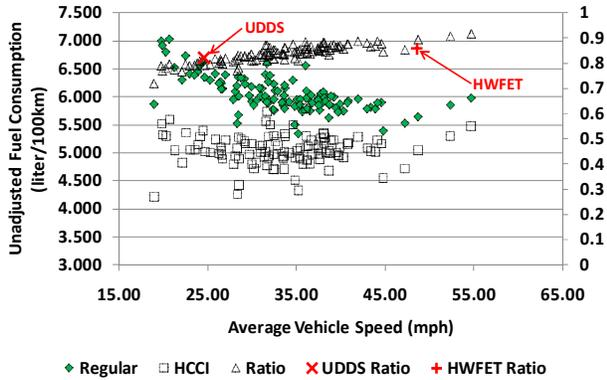
Figure 3: Fuel Consumption Impact of HCCI Technology on RWDCs for Conventional Vehicles.
