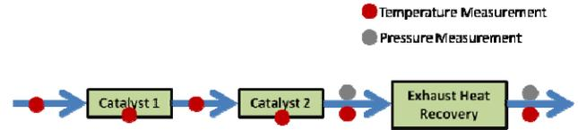
Figure 3. Exhaust System Instrumentation
