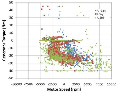
Figure 15. Electric Machine (MG1) Usage
