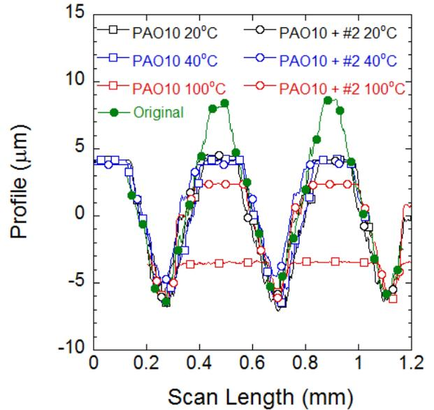
Figure 6: Wear measurements of samples tested using PAO10 and PAO10 containing 3 wt% BN/surfactant at 20°C, 40°C, and 100°C.
