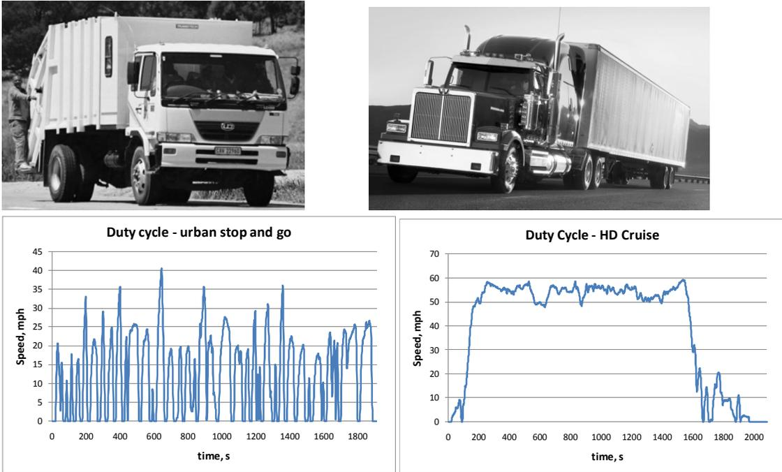
Figure 1. Comparison of typical speed cycles for two trucking applications
