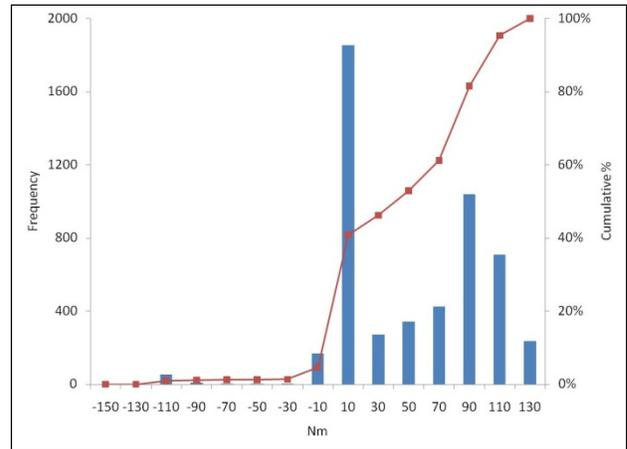
Figure 8 Brake load histogram, UDDS cycle, 266 K cold start.
