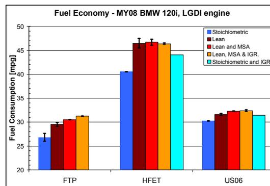
Figure 2. Fuel Economy and its Spread as a Function of Vehicle Mode and Drive Cycle.
