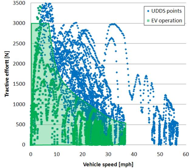
Figure 9. Electric-only Operation Area Overlaid with Urban Cycle Operating Points
