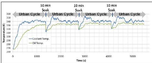
Figure 16. Coolant and oil temperature recorded over repeated UDSS cycles.
