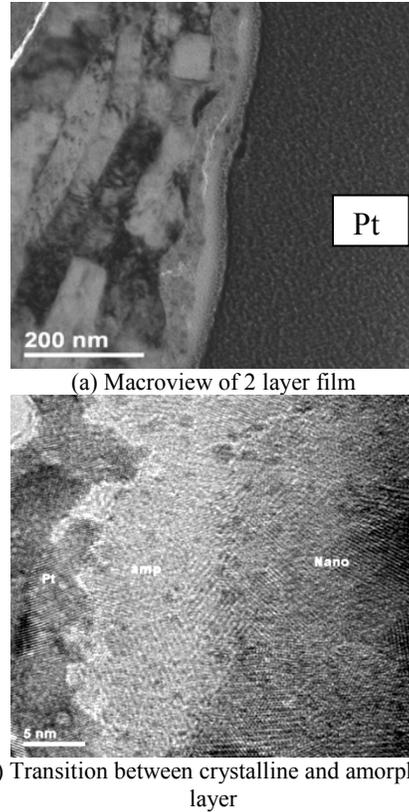
Figure 3: Tribochemical films from lubricant B is bi-layer.
