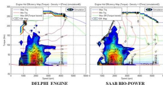
Figure 5. Conventional vehicle engine speed histograms (UDDS)
