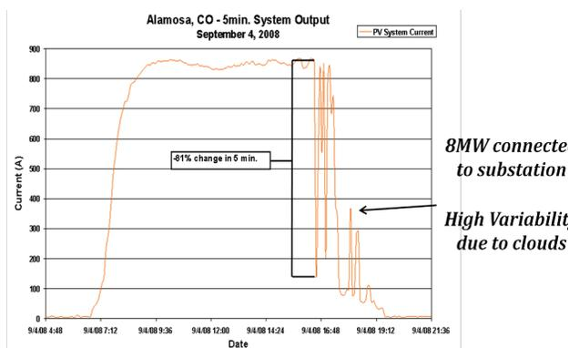
Figure 3. Cloud Patterns Create Fast Dynamics in Solar Generation
