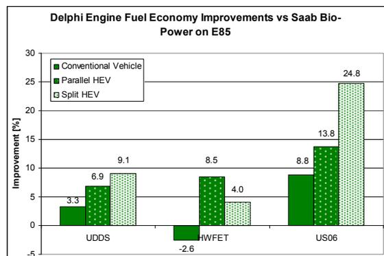
Figure 4. Relative fuel economy improvement obtained by the ethanol-optimised engine compared to the Saab Bio-Power engine
