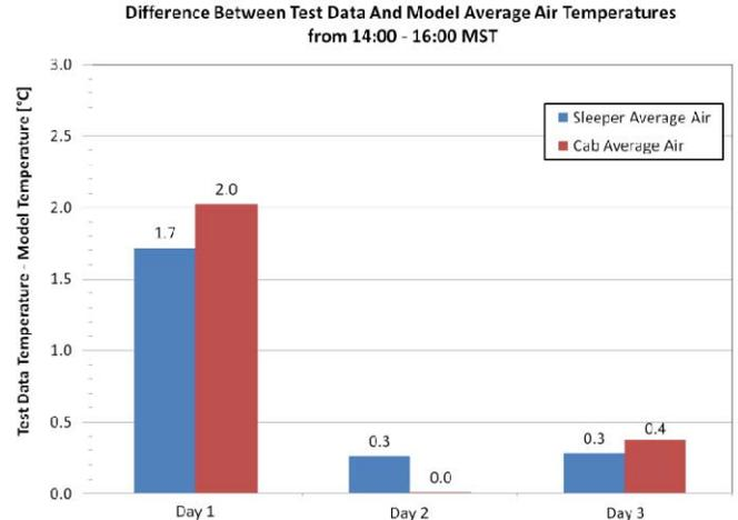
Figure 19. Comparison of Test Data and Model, Time Average from 2-4 pm
