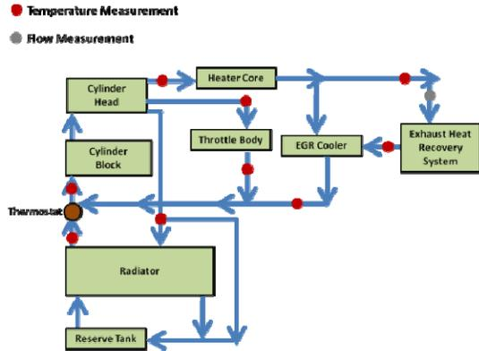
Figure 1. Main Cooling System Overview and Thermocouple Placement.
