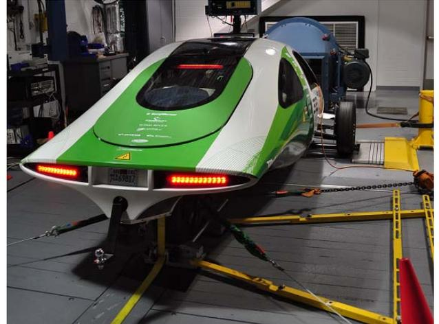
Figure 6. Team Aptera (#32) testing on the dynamometer
