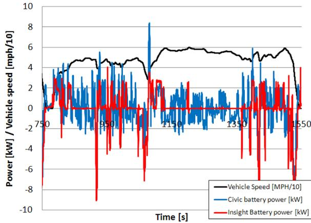
Figure 5. Usage of Hybrid System of an Insight Compared with a Civic Hybrid
