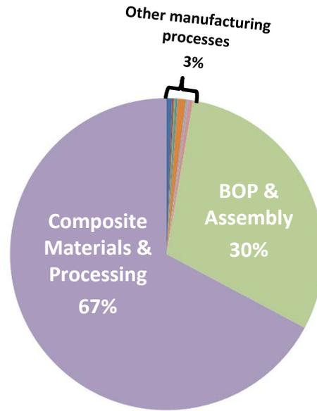
**Figure 4. Percent Cost Breakdown of a 700 bar Type IV Hydrogen Storage System at 500k Units per Year<sup>18</sup>**
