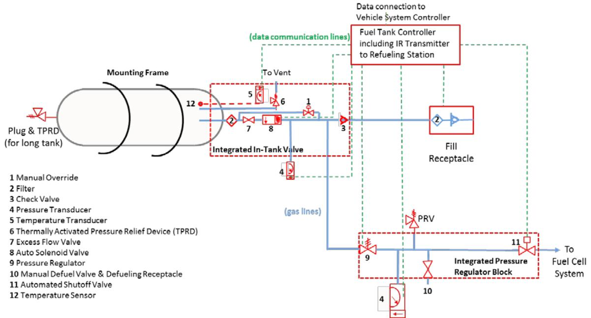
Figure 1a: Example 700 bar Hydrogen Storage System Diagram Showing a Single-Tank Configuration<sup>7</sup>
