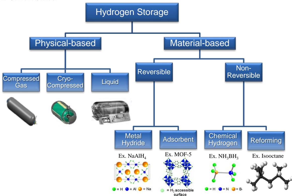
**Figure 3. Potential Hydrogen Storage Technologies**
