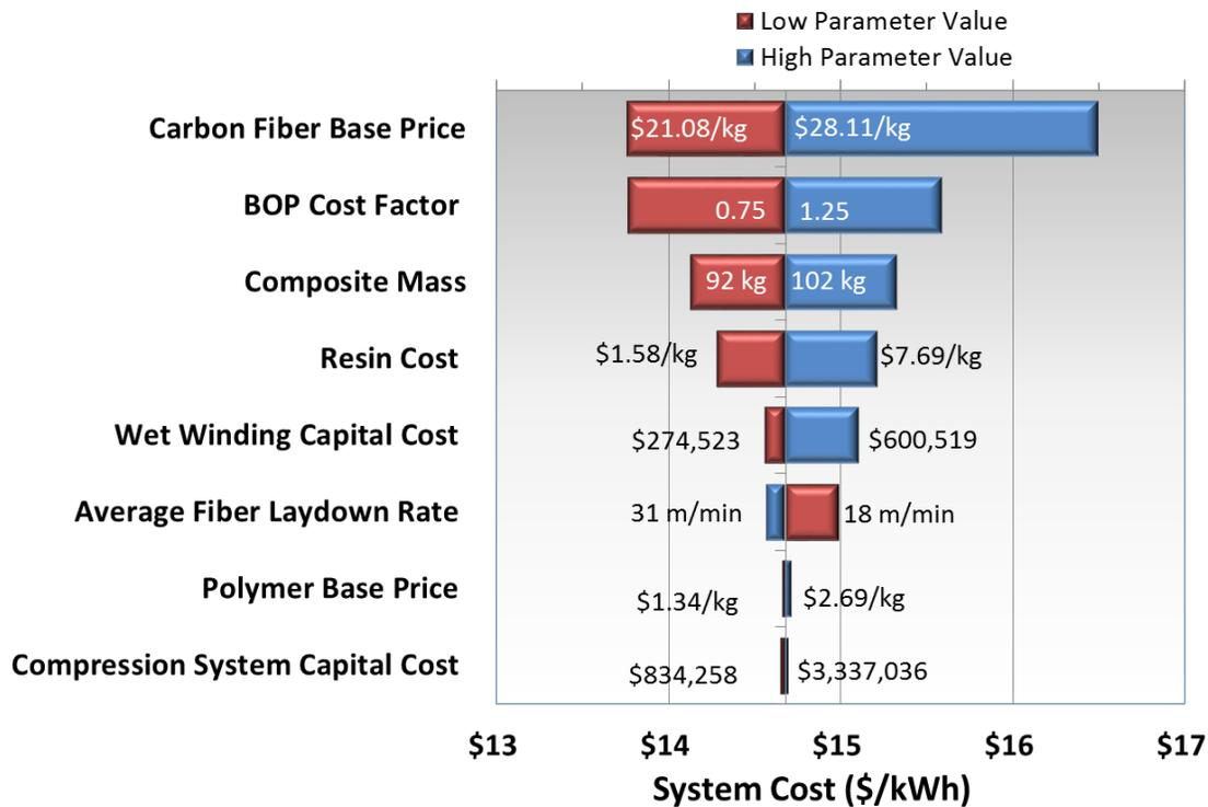
**Figure 6. Single Variable Sensitivity Analysis of 700 bar Type IV Hydrogen Storage Systems<sup>16</sup>**
