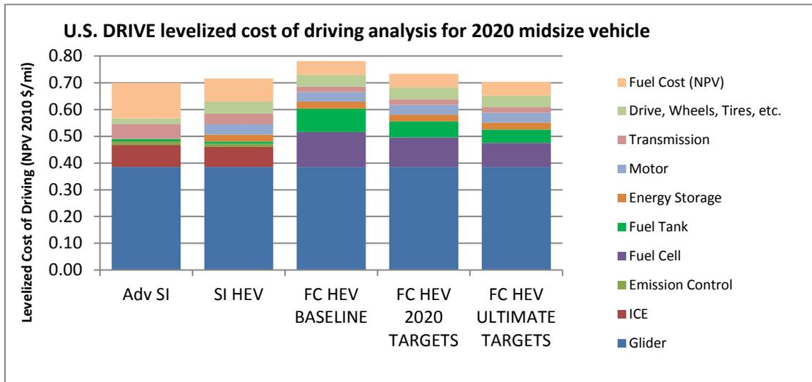
Figure 2: Levelized Cost of Driving Analysis for a FC HEV with baseline, 2020 targets, and Ultimate Target Assumptions in Comparison to Adv SI and SI HEV to establish the Onboard Hydrogen Storage System Cost Targets
