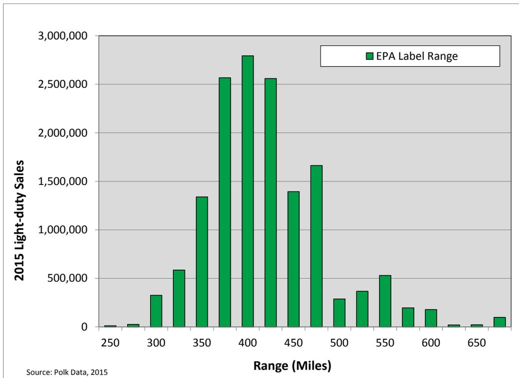
**Figure 2: Distribution of 2015 Light-duty Vehicle Sales in the U.S. Market by Driving Range (based on the product of the EPA combined fuel economy and rated fuel tank capacity)<sup>2</sup>**
