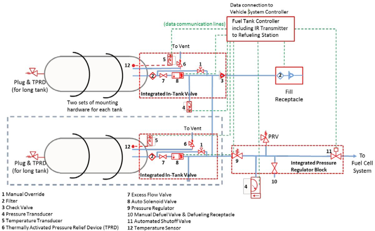
Figure 1b: Example 700 bar Hydrogen Storage System Diagram Showing a Dual-Tank Configuration
