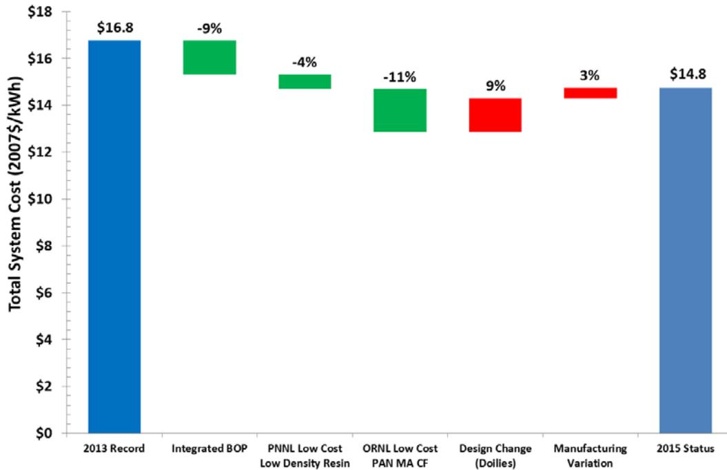
**Figure 5. Cost Reduction based on DOE Hydrogen Storage Program supported R&D compared to the 2013 baseline for 700 bar, Type IV Hydrogen Storage Systems<sup>16</sup>**
