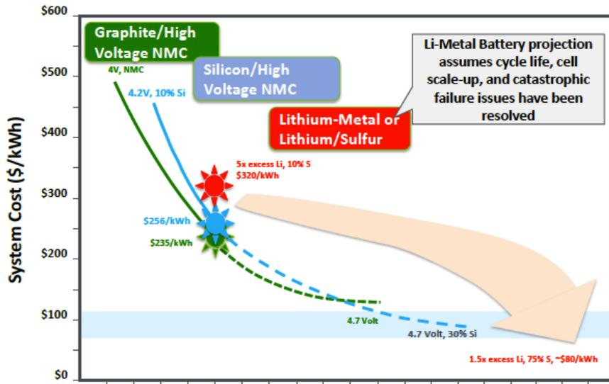
Figure 2. Potential cost trends for Li based EV batteries.
