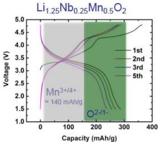
**Figure 8. Charge discharge curves a disordered and lithium rich material. Research from the Ceder group at UC Berkeley.**
