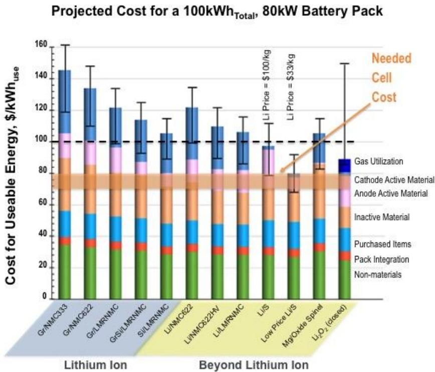
**Figure 1. Next Gen Li-ion and BLI Chemistry Cost Estimates with no XFC capability**
