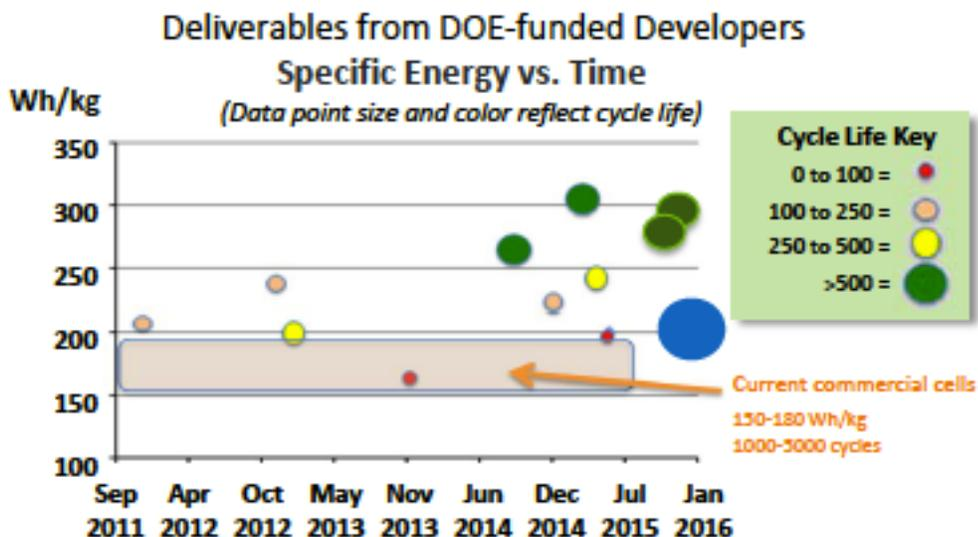
**Figure 7. Specific energy and life of silicon containing cells**
