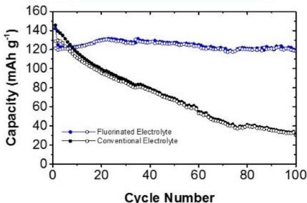
**Figure 9. Capacity retention of  $\text{LiNi}_{0.5}\text{Mn}_{1.5}\text{O}_4$ /graphite cells cycled at  $55^\circ\text{C}$ , from 3.5–4.9V, with F-electrolyte compared with conventional electrolyte at C/3 rates. (Research from the Zhang group at ANL).**
