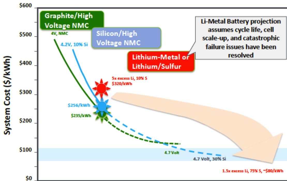
The potential Electric vehicle battery cost decrease over time, assuming successful research results in three technology areas
