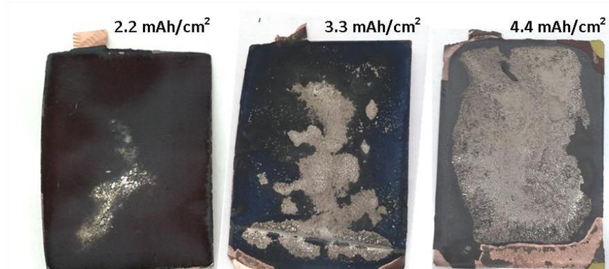
**Figure 10. Images of graphite electrode in NMC622/Gr pouch cells. Lithium plating appears as metallic deposits on the surface of the electrode. Research from the Bloom group at ANL.**
