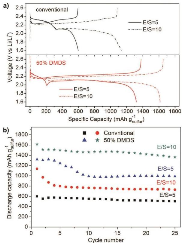
Figure 4. Electrochemical performance of high-sulfur-loading cathode with low electrolyte to sulfur (E/S) ratios of 10 and 5 mL g<sup>-1</sup> in conventional and DMDS-containing electrolytes. Research from the Wang group at Pennsylvania State University.
