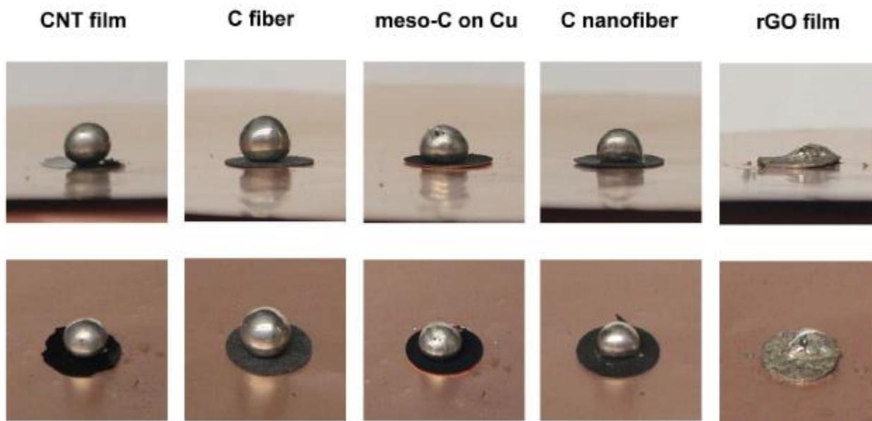
Figure 5. Example of various carbons' ability to incorporate Li metal. r-GO is being used as a Li-metal host. Research from the Cui group at Stanford University.
