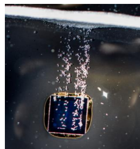
Figure 1. H 2 bubbles being generated in water from the illumination of a high-efficiency semiconductor-based PEC cell.
