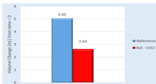
Figure 1. Li-ion NMC pouch cell battery. Reference cell represents a standard battery. Ref. +OS3 contains 2% OS3 material. Test conditions: Storage at 60°C, 10 weeks.
