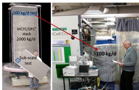
Figure 1. Relative size of FCE's production MCFC/DFC ® cell and stack capable of 2,000 kg H 2 /day operation and sub-scale test cell and 100 kg H 2 /day stack used in the project.
