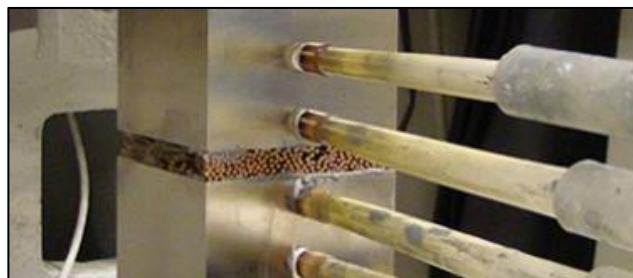
Figure 1. Test specimens with thermal transmittance setup for thermal measurements perpendicular to the wire axis.
