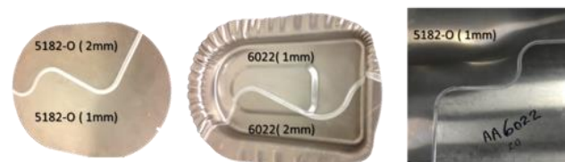
Figure 2. Curvilinear welds made between (a) AA5182-O (1 mm-2 mm), (b) AA6022-T4 (1 mm-2 mm), and (c) AA5182-O (1 mm) to AA6022 (2 mm).
