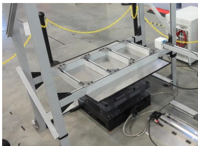
Figure 1. INL's test apparatus enables interoperable performance testing of WPT systems off-board the vehicle. Testing conducted by INL provides detailed results to support the development and harmonization of WPT codes and standards
