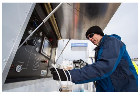
Figure 1. NREL researcher Chris Ainscough prepares HyStEP for testing at NREL's Energy Systems Integration Lab. (Photo by Dennis Schroeder/NREL.)
