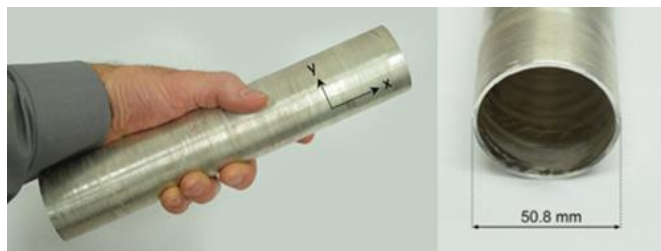
Figure 2. A 30 cm length of ZK60 tubing extruded using the ShAPE process along with a cross section showing the 1.52 mm nominal wall thickness.
