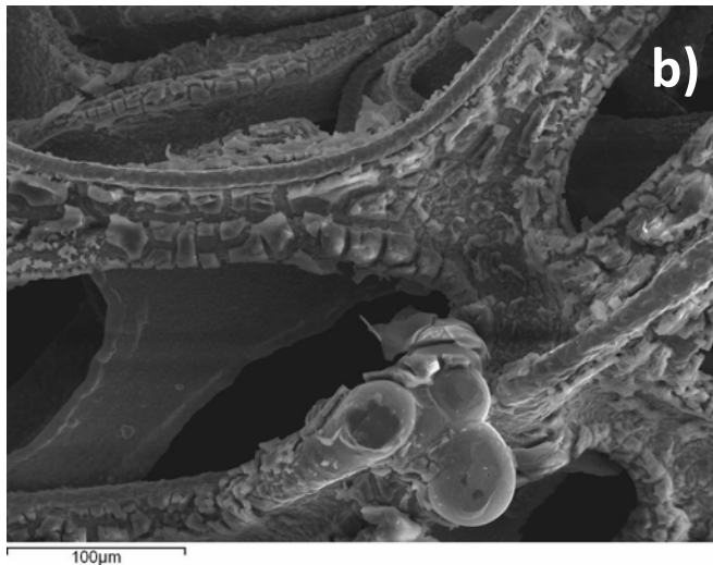
SEM micrographs of electrodeposited silicon a) on synthesized copper foam, pore sizes \sim 50\mu\text{m} b) on commercial foam (calendared), pore sizes \sim 300\mu\text{m}
