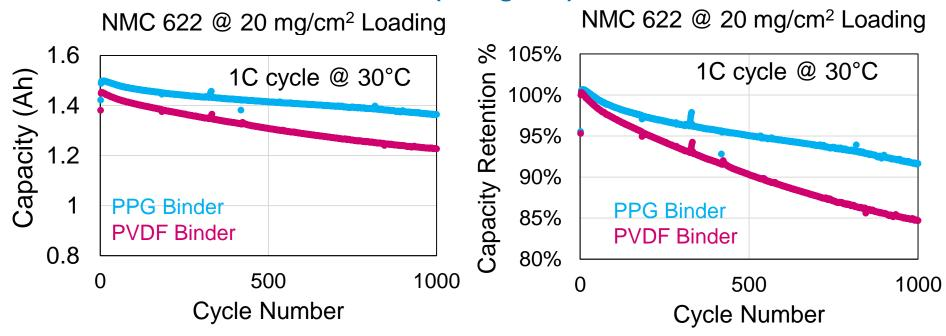
Cells with PPG binder significantly outperformed cells with PVDF-NMP binder
