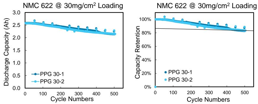
Cells with PPG binder significantly outperformed cells with PVDF-NMP binder
