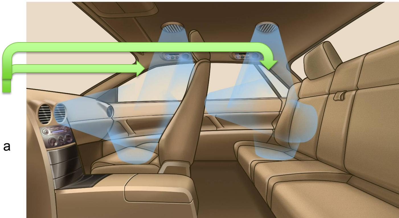
Zonal TE units located in dashboard, headliner, A&B pillars and seats/seatbacks
