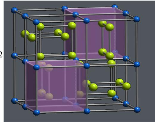
*Atoms can be inserted into empty sites. Atoms can “rattle” in these sites – scatter phonons and lower the lattice thermal conductivity.*
