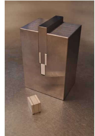
Double-Lap Shear Fixture and Sample
