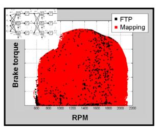
Extensive engine mapping is used in neural network model training
