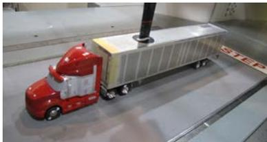
Transition to new 1/8<sup>th</sup> scale, rolling-road wind tunnel facility-moving belt better simulates vehicle moving down the road
