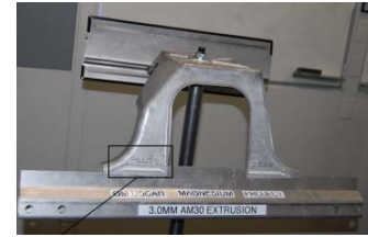
Joining demonstration: laser assisted (left) self piercing rivet and FSW (right)
