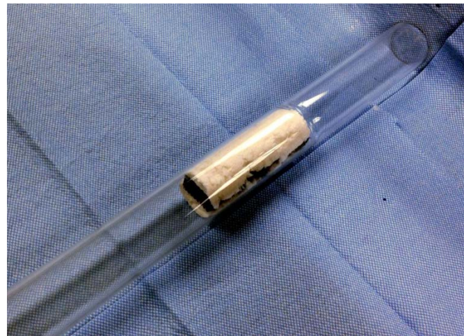
Sample of GTI catalyst inserted in reactor tube
