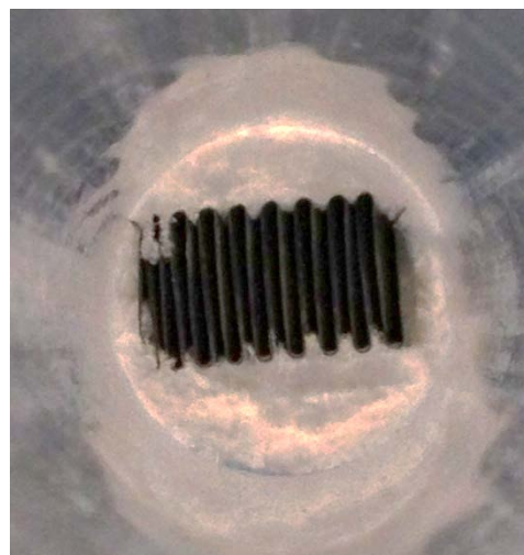
Sample of GTI catalyst inserted in reactor tube
