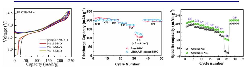
(Left) 1<sup>st</sup> cycle behavior of NMC811 in voltage range 2.8-4.6 V; (middle) rate capability of NMC811 with a LiBO<sub>2</sub>/LiF coating in voltage range 2.8-4.6 V, and (right) rate capability of LiNi<sub>0.94</sub>Co<sub>0.06</sub>O<sub>2</sub> after storage in voltage range 2.8-4.4 V.
