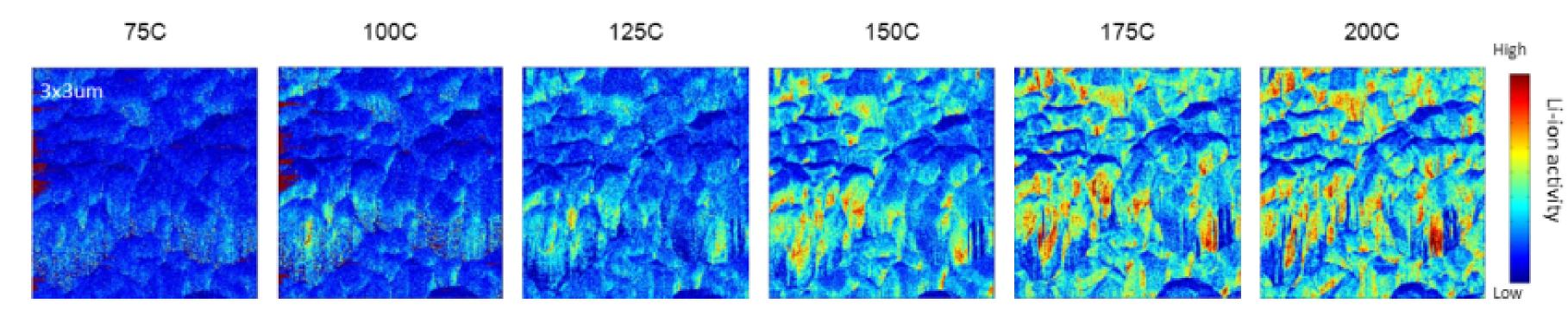
The temperature-dependent ESM signal for each individual pixel show linear curves in Arrhenius-type plot. From the slope, we can extract spatially resolved maps of the activation energy (after image alignment and Gaussian filter application to reduce pixel-to-pixel noise).
