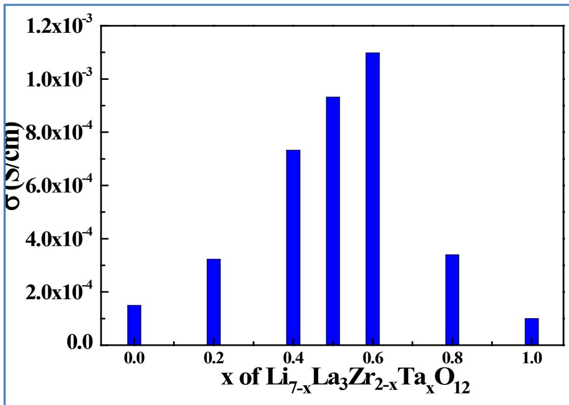
In accordance with prior result results, a maximum  $\sigma_{\text{Li}^+} > 10^{-3} \text{ S cm}^{-1}$  has been obtained at  $x=0.6$  (nominal composition  $\text{Li}_{6.4}\text{La}_3\text{Zr}_{2.4}\text{Ta}_{0.6}\text{O}_{12}$ ).
