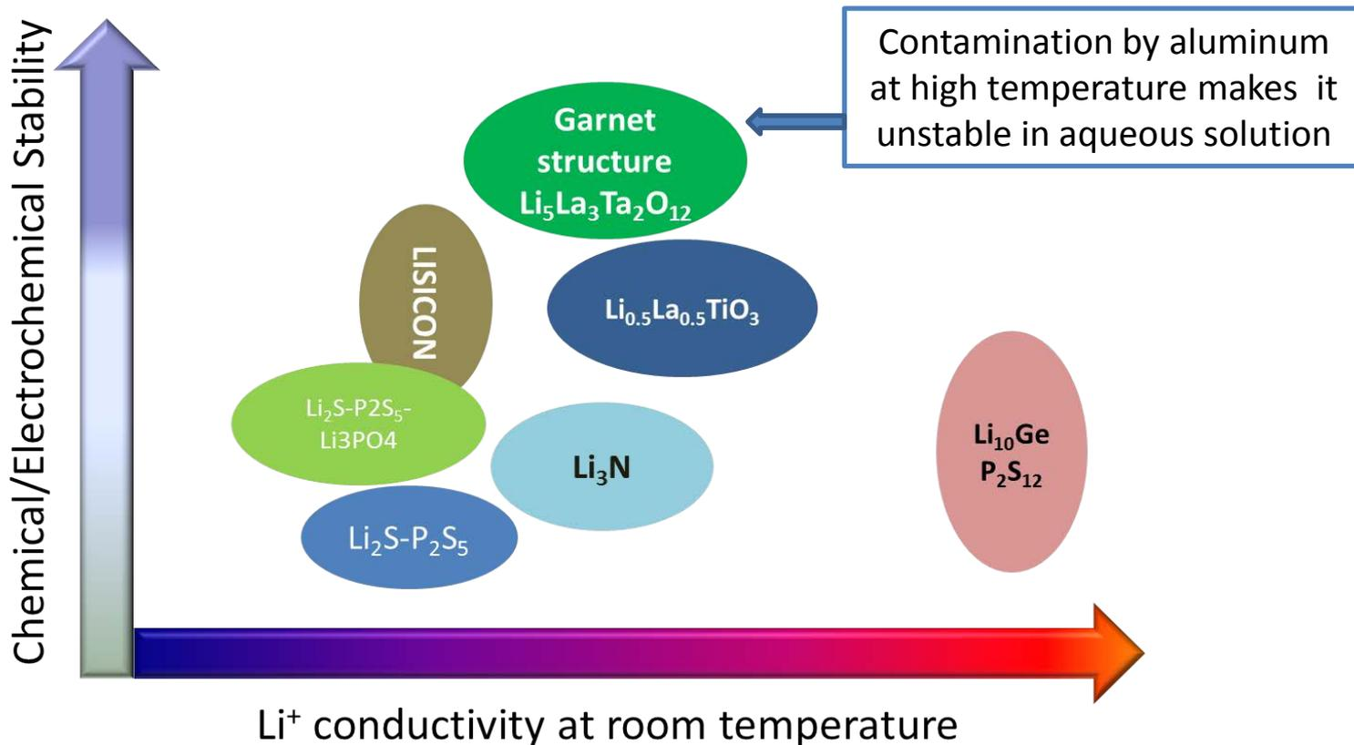
Garnet structure electrolytes are electrochemically stable with a larger window than commercial LISICON<sup>®</sup> membrane and are not sensitive to water as sulfides, so they are a promising separators for flow-through batteries using aqueous solutions.
