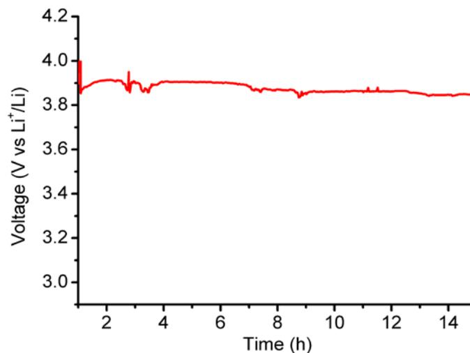
Garnet solid electrolyte is stable in bromine carbonate solution
