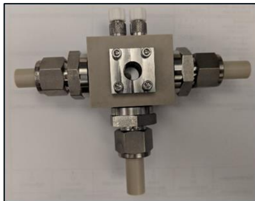
O-ring 3-electrode cell to control surface exposure
