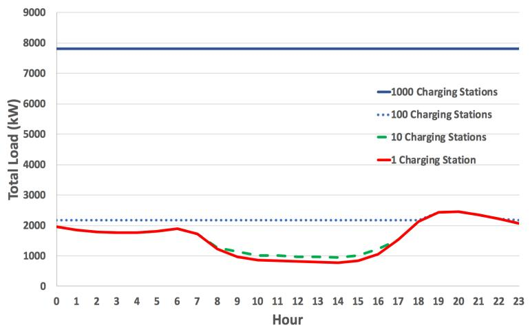
1000 CS approach max load. 100 CS show valley filling. 1 or 10 CS have negligible effect. Net Load from 6—10pm cannot be flattened by reducing charge load.
