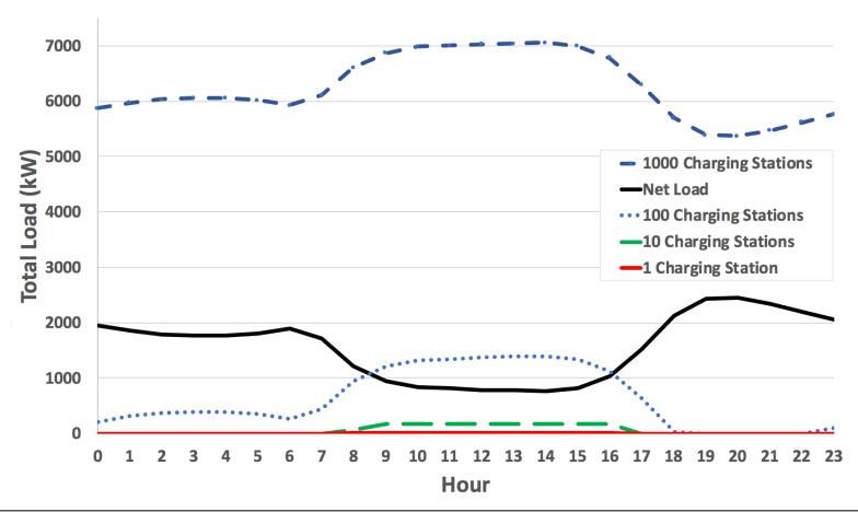
Net Load model based on CAISO data. Total demand limited to 8000 kW (kilowatts). Each charging station serves 3 PEV, and can draw 18kW max.
