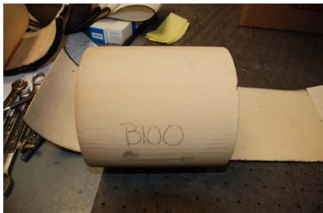
Figure 5. Surface of the DPF after being exposed to B100 exhaust and storage for 3 months in order to simulate the original DPF degradation.
