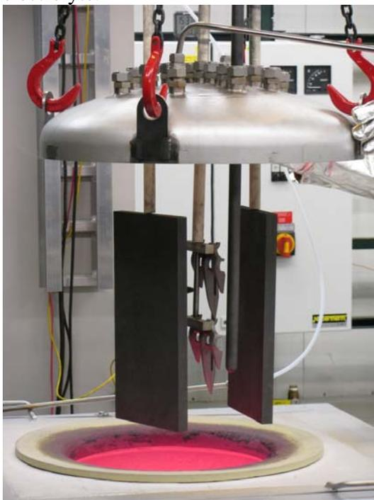
*Figure 2. View of 22 in. boriding unit. Some industrial parts ready to be immersed into the molten electrolyte.*
