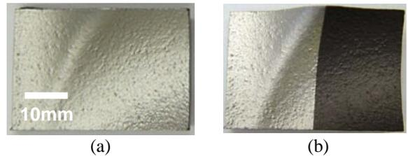
**Figure 2.** Photographs of TBC specimen #10 with (a) as-received and (b) a black-painted surface.
