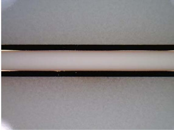
Figure 15. Polished cross-section of a DBC with 1.02-mm thick Al<sub>2</sub>O<sub>3</sub> sandwiched by 0.30-mm thick copper cladding.
