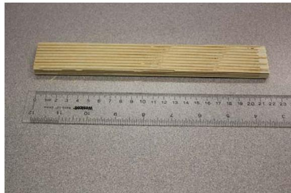
Figure 4. Example of a sectored flexure bend bar harvested from a DPF. Intended for 4-pt bend testing.
