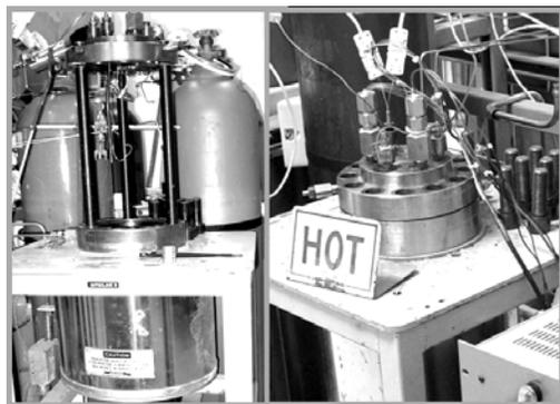
**Figure 3.** High-pressure hydrogen autoclaves used to charge piezoelectric samples
