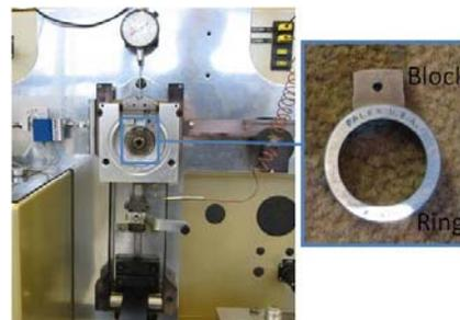
Figure 2. Conformal block-on-ring test rig for simulating journal bearing application
