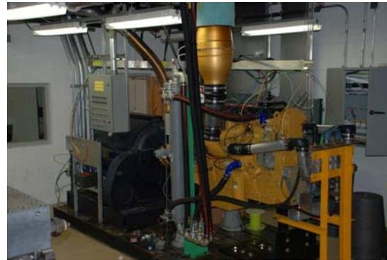
Figure 1. Photograph showing mounted engine and dynamometer. Engine has been instrumented for 2<sup>nd</sup> Law Analysis.
