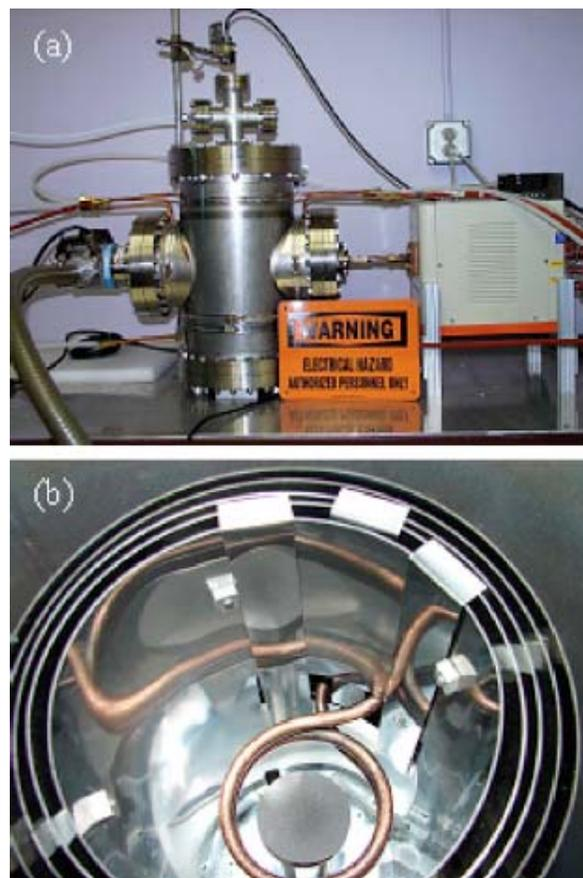
Fig. 1. Photograph of the high temperature induction furnace
