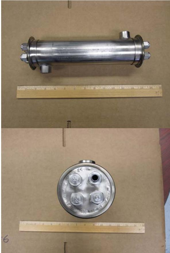
Figure 2: Two views of the tube reactor that will be used to generate deposit samples.
