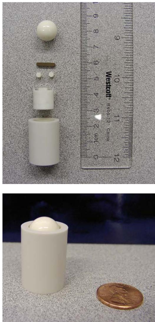
Figure 3. Self-aligning, high-temperature (all-alumina) three-point-bend fixture used to measure flexure strength of 1.5 mm x 1.5 mm x 12 mm prismatic bars. Bend span is 8 mm. Exploded (top) and assembled views (bottom).
