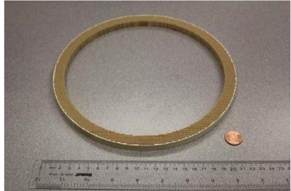
*Figure 6. Example of an o-ring specimen harvested from a DPF. Its interior provides the interior-disk specimen shown in Fig. 3. Intended for diametral compressive testing.*
