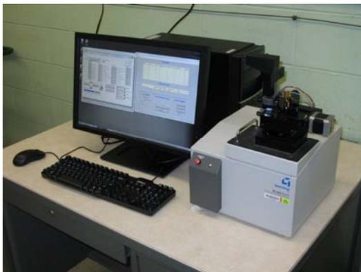
Figure 2. Computer controlled scratch tester for coating adhesion energy measurements.
