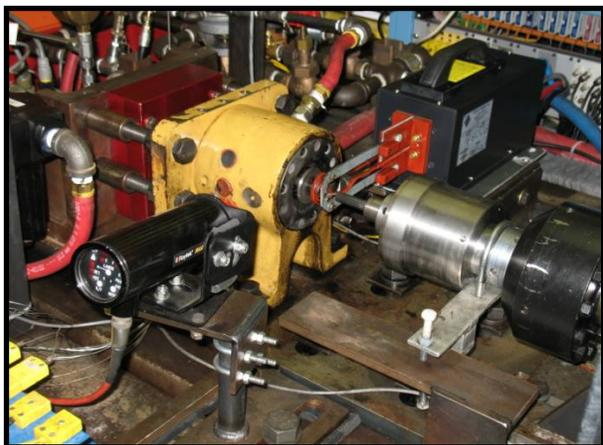
**Figure 1.** Buettner Rig engine simulation facility for testing high-temperature wear and performance of exhaust valves and seats at the Caterpillar Technical Center.
