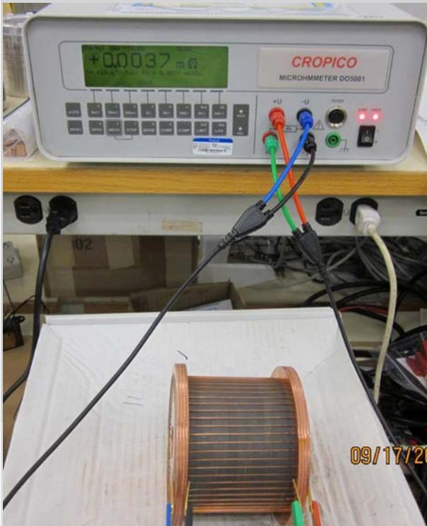
Figure 5. Electrical resistance testing of the rotors at GM. Electrical clamps are connected, one on each end cap, across a bar.
