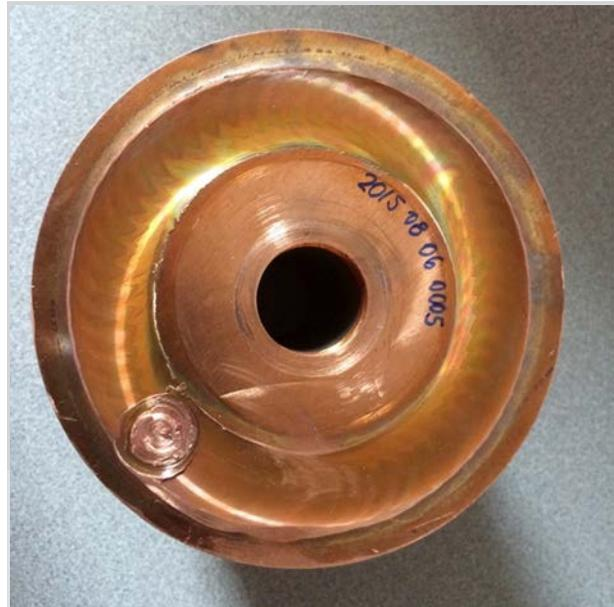
Figure 4. FSW full-size rotor end cap.
