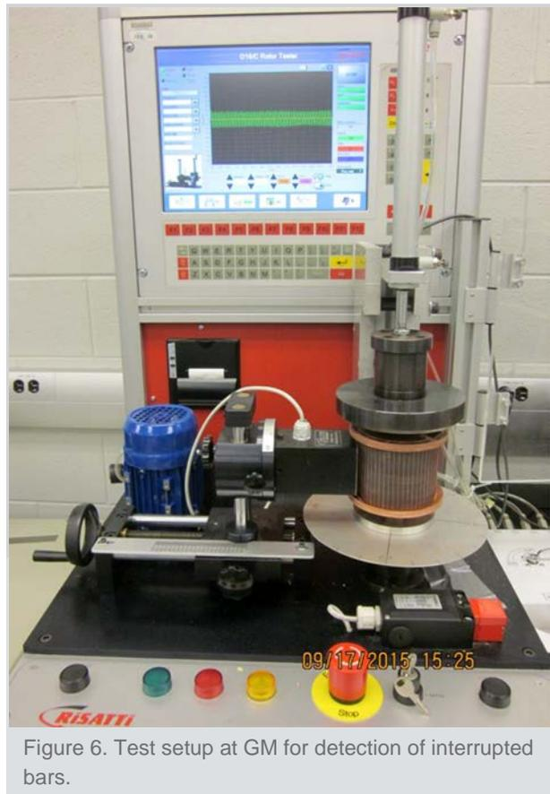
Figure 6. Test setup at GM for detection of interrupted bars.
