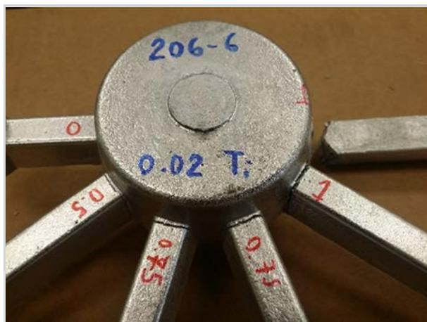
Figure 48. An image of the casting for evaluation of susceptibility to hot tearing.
