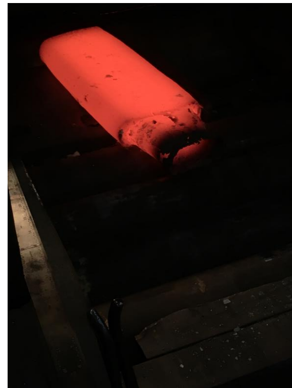
Image of 50 lb heat of ORNL chromia-forming alloy being successfully hot rolled at Special Metals
