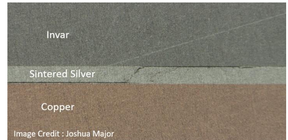
Cross-sectional image of cracks formed in sintered silver bond under thermal cycling: sintering pressure – 3 MPa; bond diameter – 16 mm
