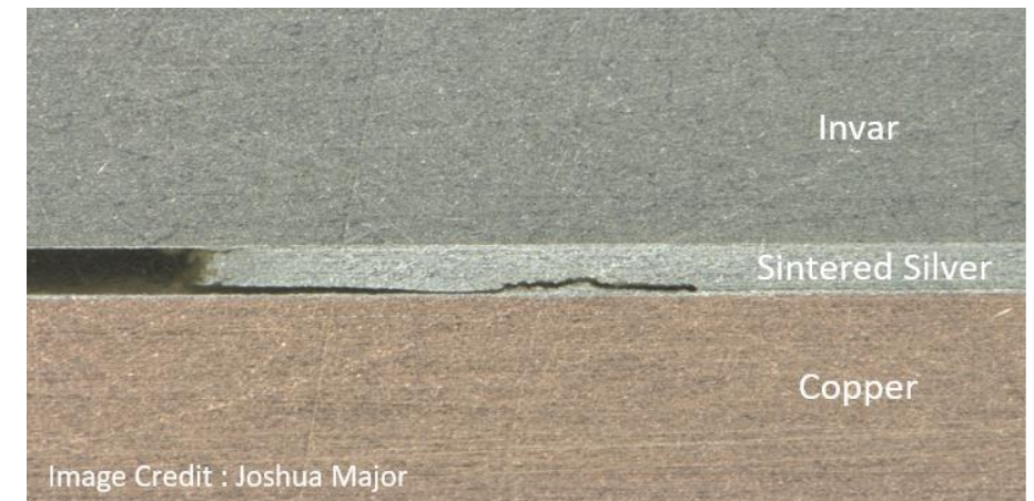
Cross-sectional image of cracks formed in sintered silver bond under thermal cycling: sintering pressure – 10 MPa; bond diameter – 10 mm
