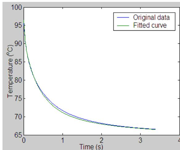
Junction temperature cooling down curve
