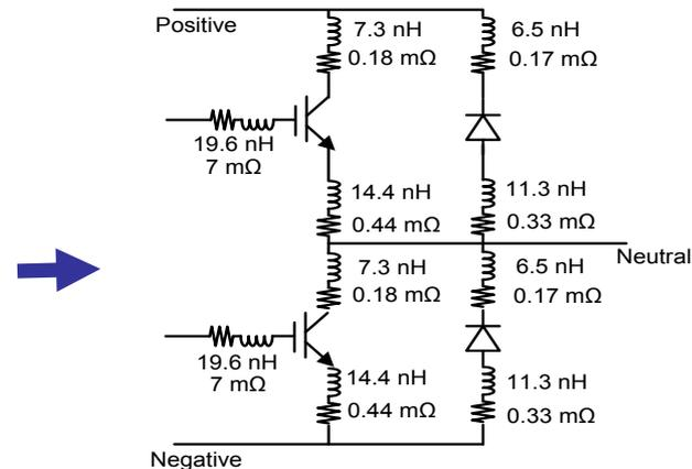
Lump element model of parasitic electric parameters
