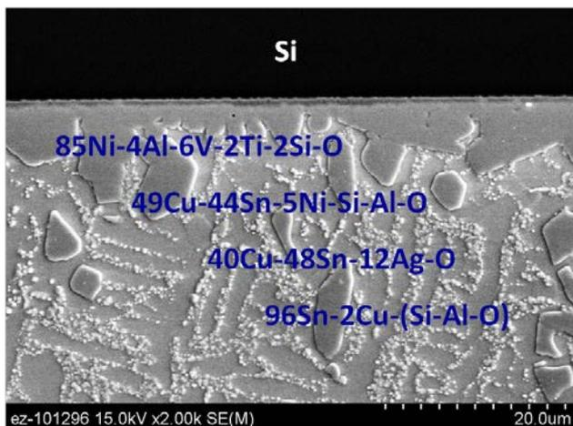
Die attach solder layer in Infineon HP1
