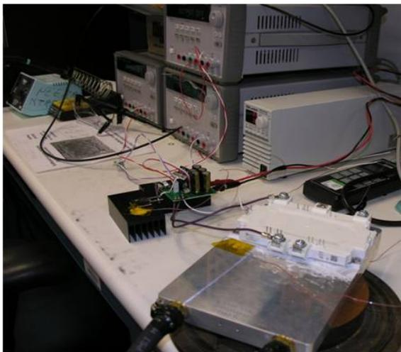
Infineon® HybridPack1™ under test
