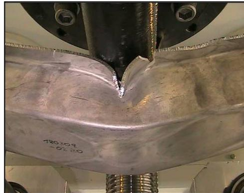
"Ductile" failure mode
