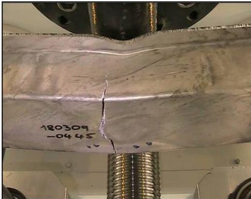
7 "Brittle" failure mode
