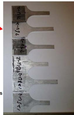
Failed tensile samples
