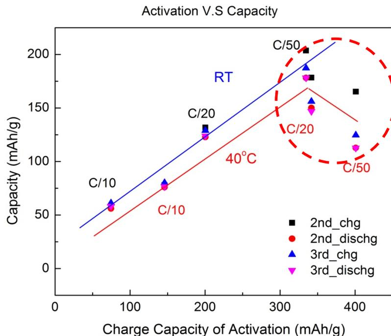
However,  $\text{Li}_2\text{MnO}_3$  activated at  $40^\circ\text{C}$  with C/50 shows lower capacity than one at  $40^\circ\text{C}$  with C/20 and one at RT with C/50
