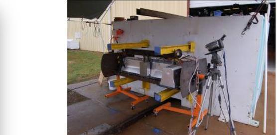
Volt battery pack being prepared for test
