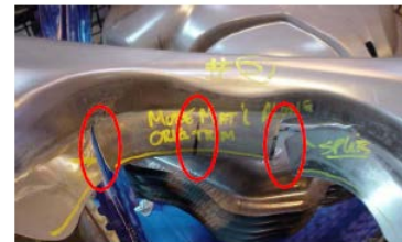
Fracture at edge during stamping, by M.F. Shi
