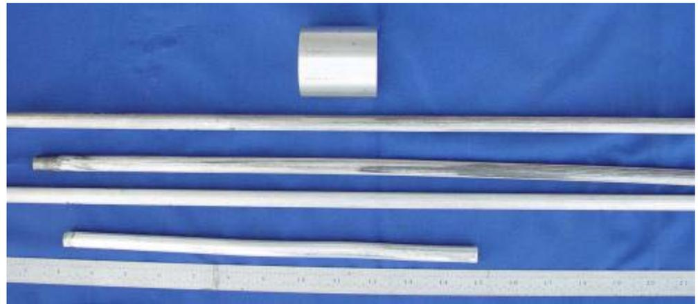
Extrusion billet (top, 50 mm diameter) shown with extruded rods. Extrusion ratio of approximately 20:1
