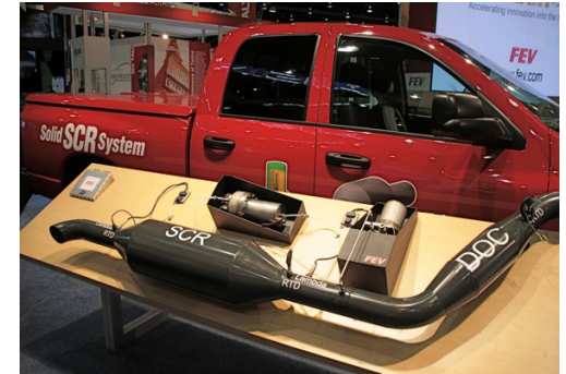
FEV solid SCR system: Ammonium carbamate
