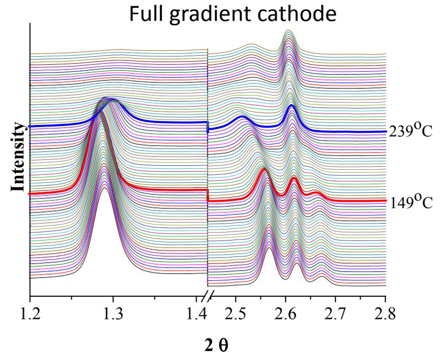
1. Mostly layered phase after cycling and heating up to 150°C
