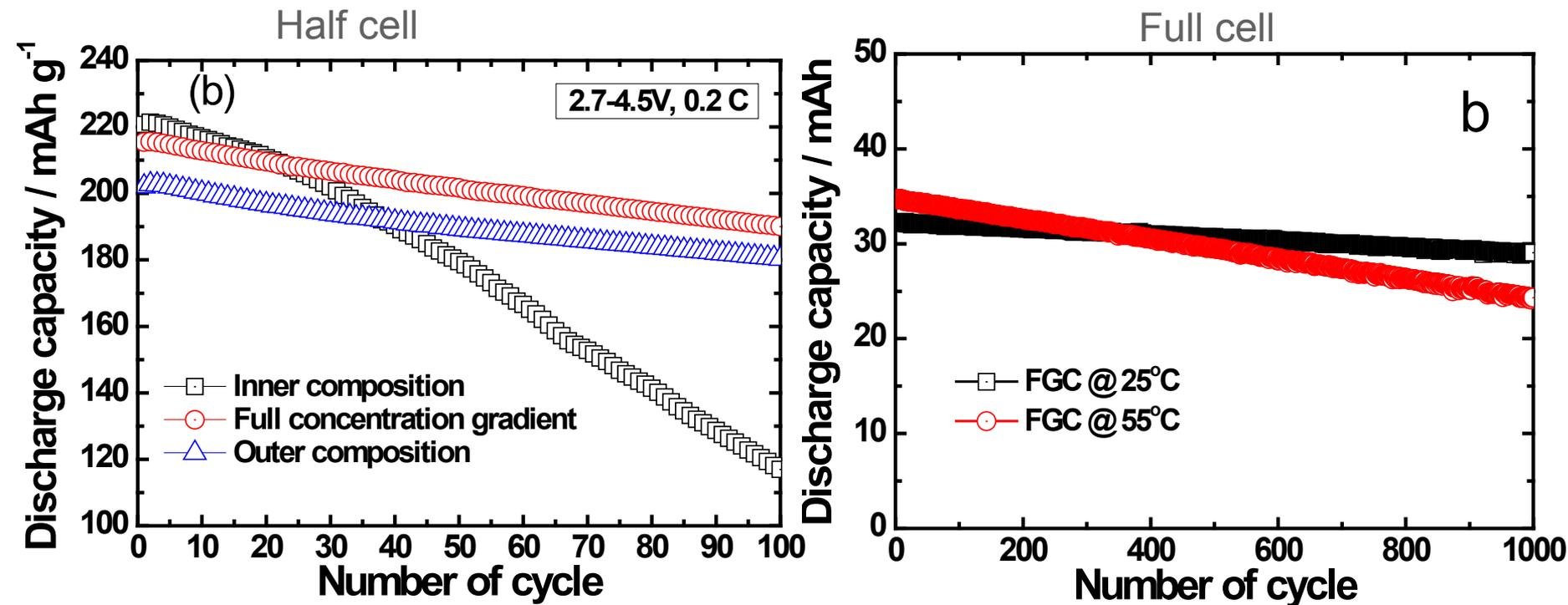
Full concentration gradient shows high capacity and very limited capacity fade after 1000 cycles at 55°C in a full cell, Electrolyte used is LiPF<sub>6</sub>/EC:EMC with 1%VC
