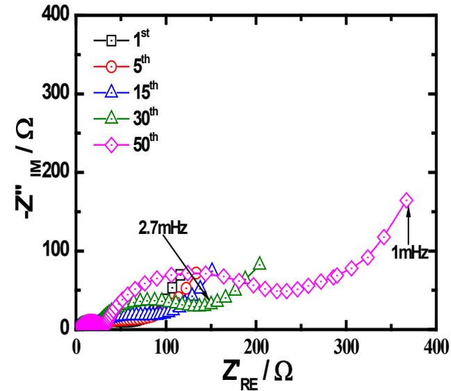
(CSCG A) with shorter shell thickness but high Mn content at the outer shell layer of the particle shows less impedance growth during cycling at 55°C.
