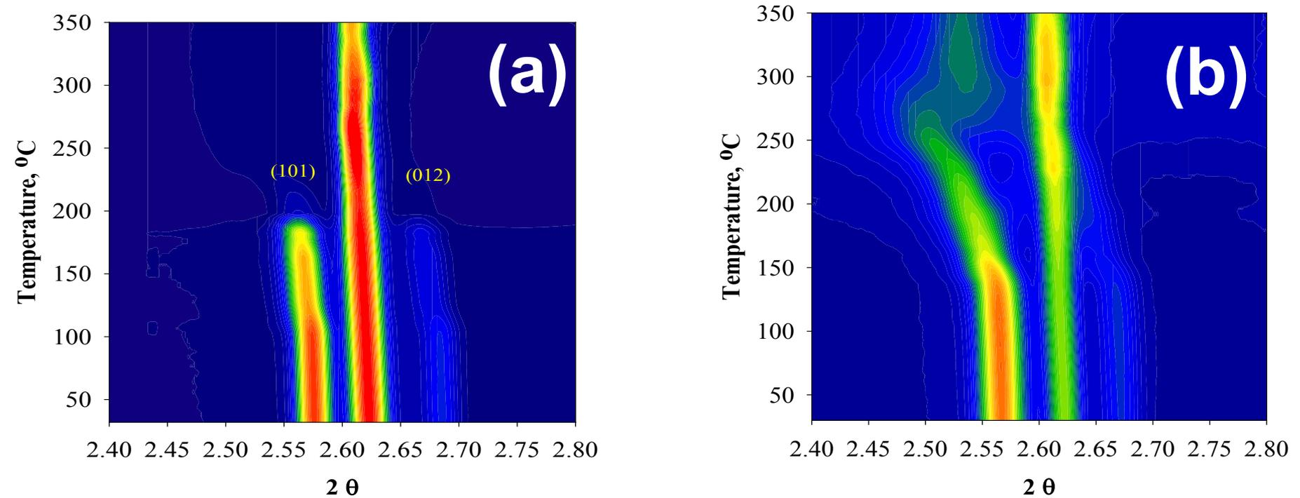
Contour plots of in situ high energy X-ray diffraction profile of (a) delithiated core composition material  $[\text{Li}_{1-x}(\text{Ni}_{0.86}\text{Co}_{0.10}\text{Mn}_{0.04})\text{O}_2]$  and (b) delithiated FGC material during thermal ramping from room temperature to  $375^\circ\text{C}$  with a scanning rate of  $10^\circ\text{C min}^{-1}$
