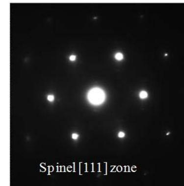
Electron diffraction of cycled core showing spinel phase
