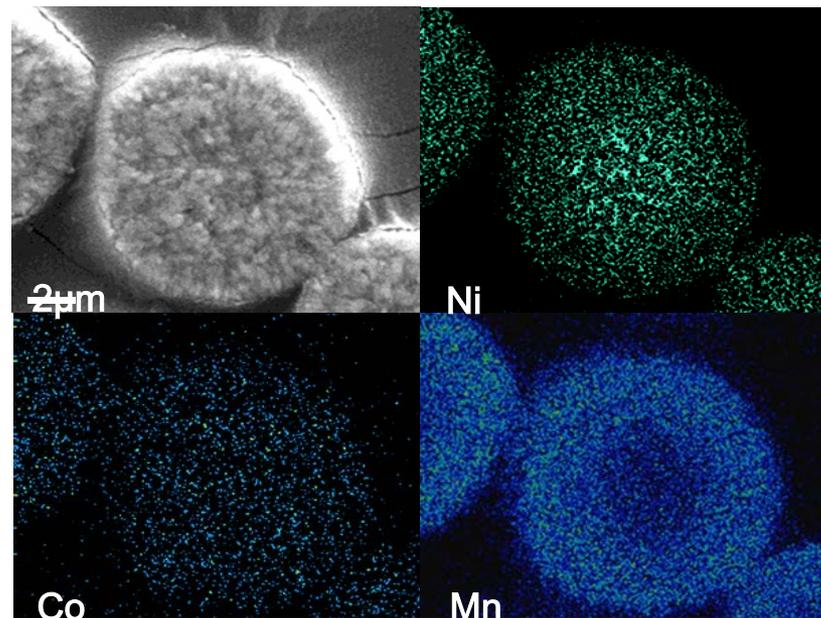
EDAX showing high concentration of Ni in the center of particle and high concentration of Mn in the outer layer of the particle
