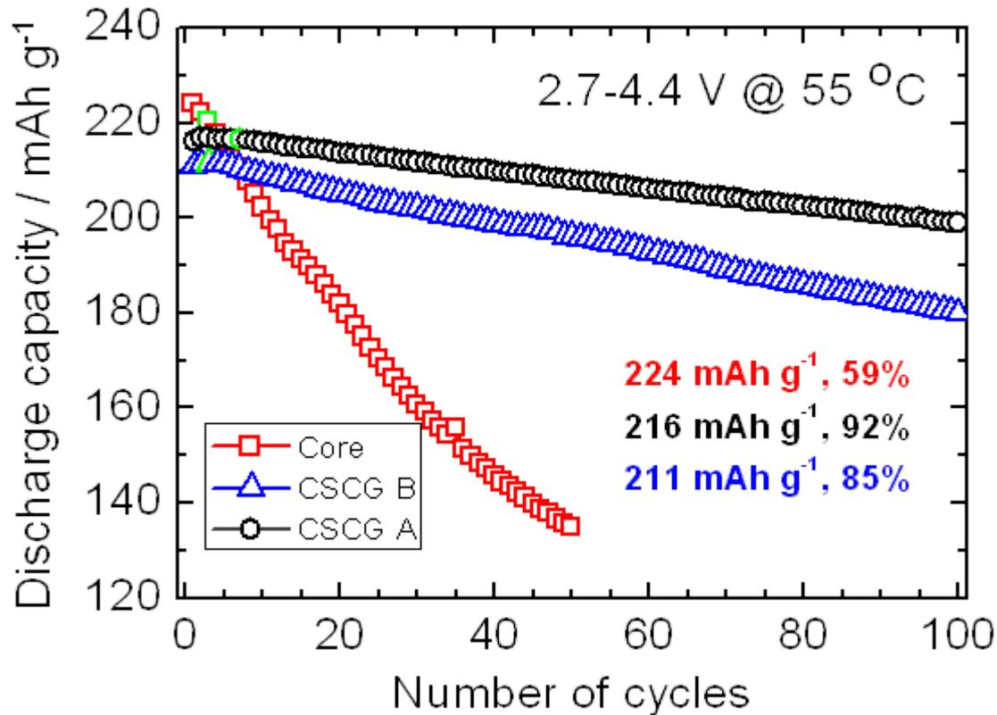
Gradient cathode that has the highest Mn content on the outer shell of the particle (CSCG A) shows better cycling performance than the one with less Mn content on the outer shell of the particles (though the later has thicker shell thickness).
