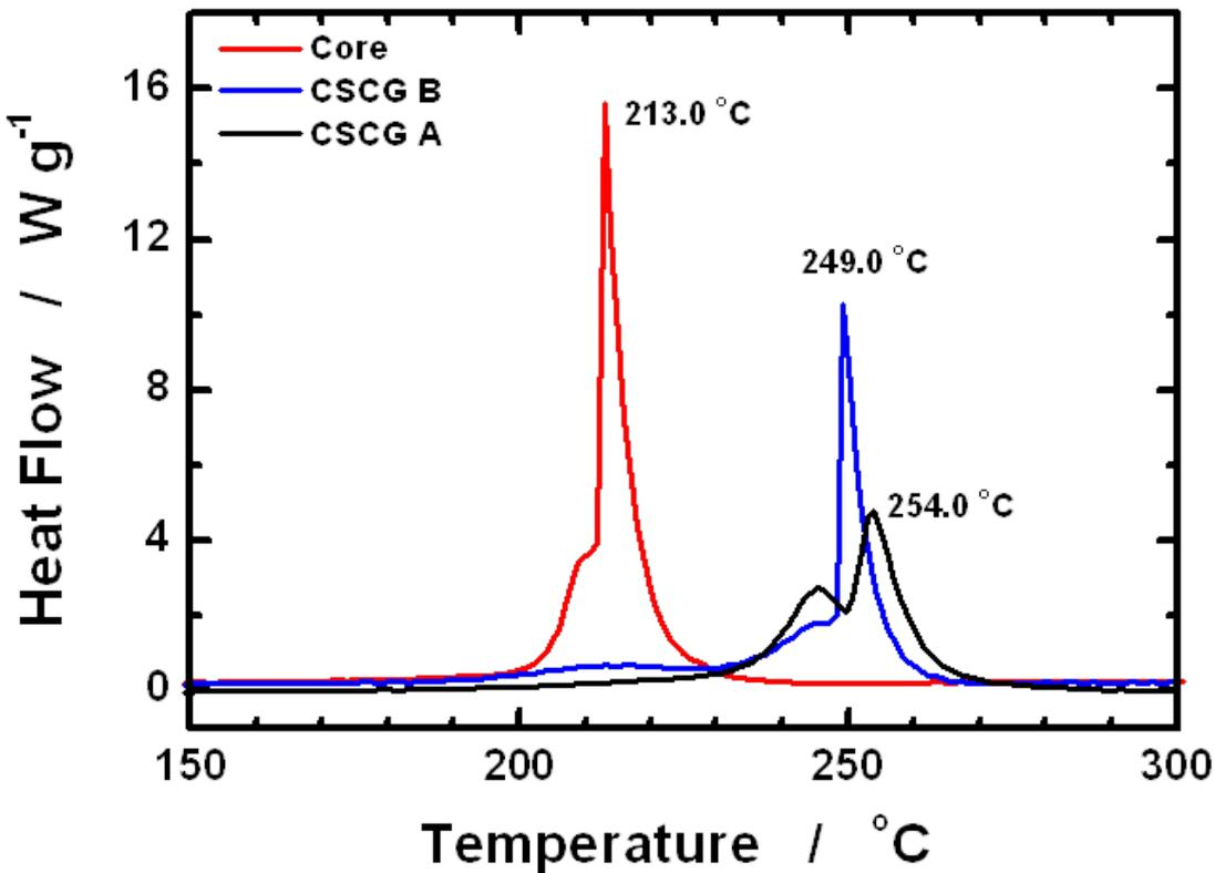
CSCGA with high Mn content at the outer shell layer shows less heat generation
