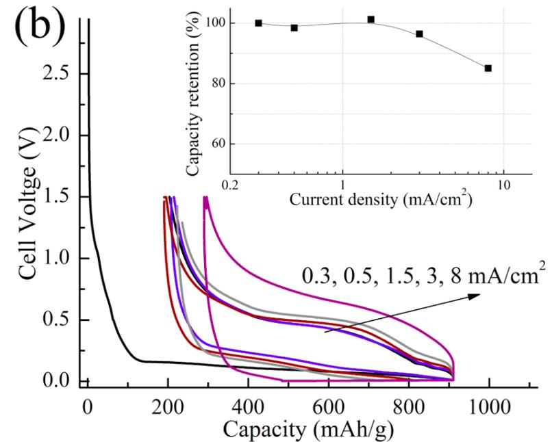
Rate capability of SMOG electrode between 0.01 V and 1.5 V. (a) capacity on cycling at different current densities; (b) cycling curves at different rates, and Ragone plot for Li insertion. 1 C rate = 2.8 mA/cm<sup>2</sup>. The first cycle current density was 0.3 mA/cm<sup>2</sup>.
