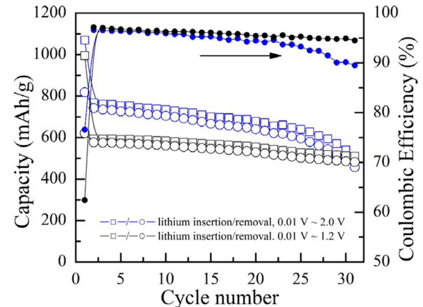
(left) XRD patterns of (A) Solvothermally formed Fe-Sn; (B) Planetary ball-milled (pBM) Sn-Fe-C composite; (C) High-energy ball-milled (HEBM) Sn-Fe-C composite. Sn metal phase in the solvothermally formed material disappears after high-energy milling with graphite. (right) Electrochemical cycling of this Sn-Fe alloy in two voltage windows; no grinding with carbon. The current was  $0.3\text{ mA/cm}^2$  in the 1<sup>st</sup> cycle and then changed to  $0.5\text{ mA/cm}^2$  thereafter.
