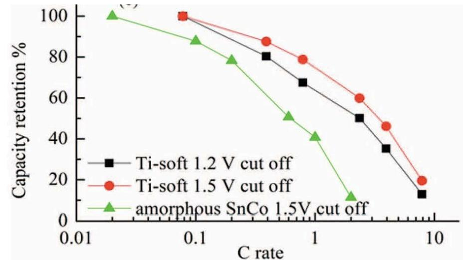
Lithium removal – discharge of cell
