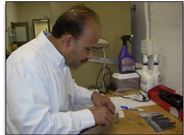
Umesh Ghandi prepares a test specimen for high strain rate tensile testing
