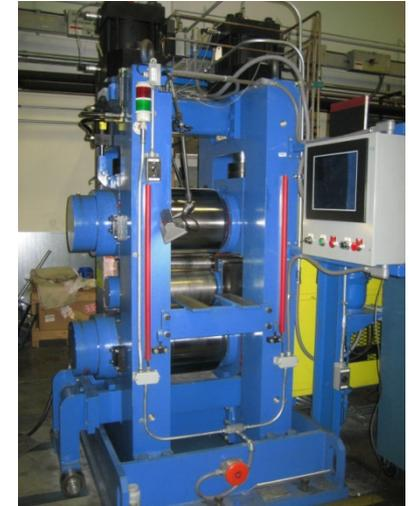
Four high mill with 3:1 sized work rolls
