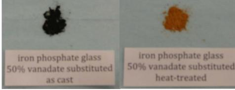
An oxygen gain of 1.9 wt.% would imply up to 48% of the iron as Fe<sup>2+</sup> in the as-cast glass (some may be due to V valence).
