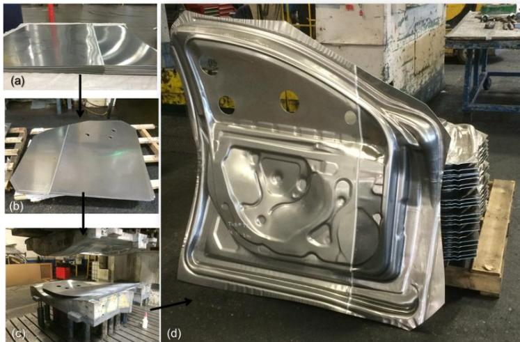
Figure III-62: Dissimilar thickness blanks produced at TWB for stamping trials showing production chain: (a) Welded blanks as produced, (b) welded blanks after laser cutting at Quality Measurement Control, Inc. (QMC Inc.), (c) laser-cut panels loaded for stamping at TWB, and (d) dissimilar thickness door inner panels after stamping showing 2-mm AA5083 welded to 1.1-mm AA5083.
