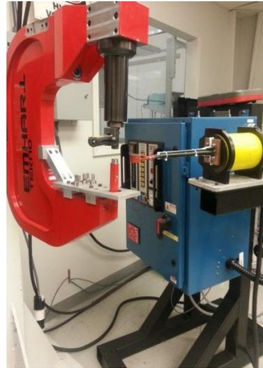
Figure III-54: PNNL's custom induction heating system integrated into Stanley's SPR system.
