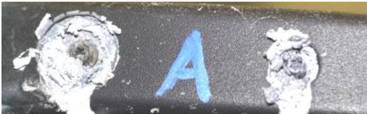
Figure V-34: Galvanic corrosion effects of steel screws in a magnesium component exposed to 240 hours of ASTM B117 salt spray testing.
