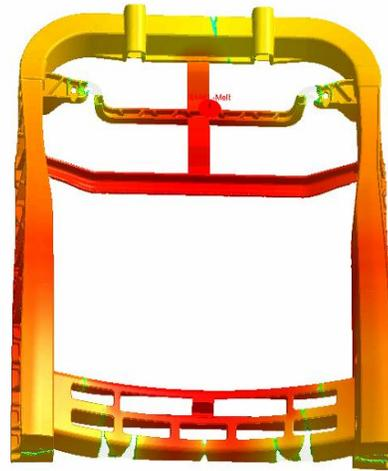
Figure IV-46: Visualization of flow time with major weld lines. Yellow indicates shorter flow times and red longer flow times which will correspond to the suspected location of weld lines.
