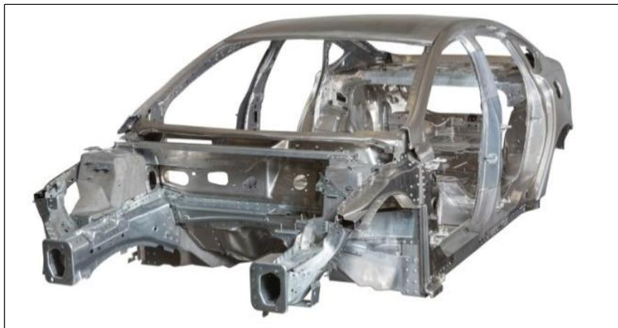
Figure V-3: Mach I BIW Prototype Build.
