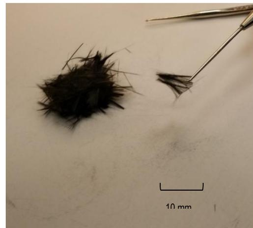
Figure IV-34: Selected PlastiComp sample showing long-entangled fibers.
