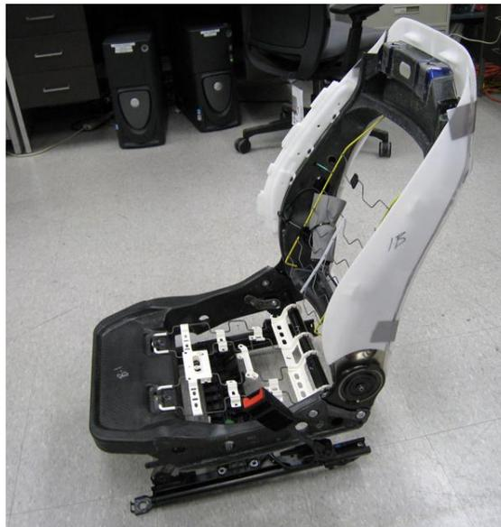
Figure V-20: CF Composite Prototype Seat.
