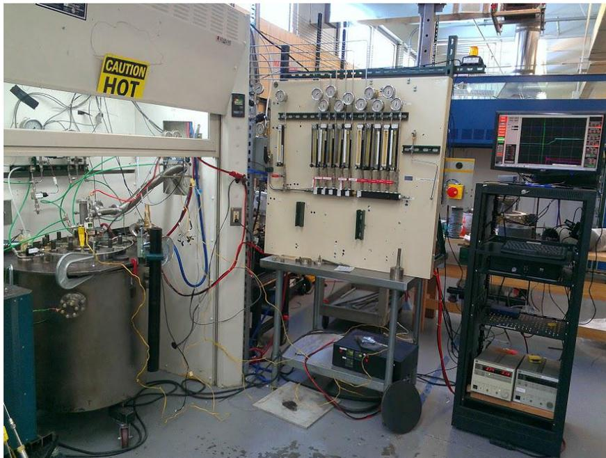
Figure III-15: Alpha prototype furnace (left) with gas panel (center) and control computer (right).
