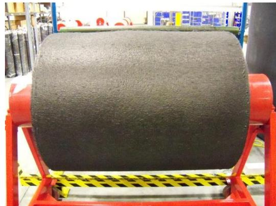
Figure IV-23: Typical roll of nonwoven roll goods material made from reclaimed CF.
