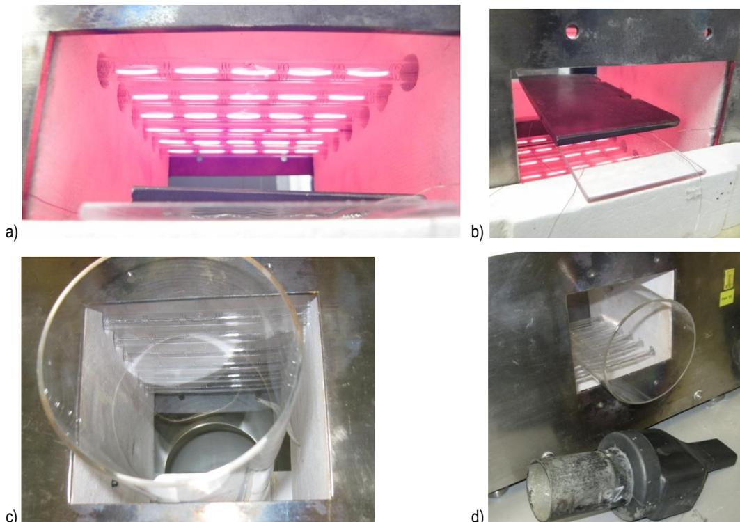
Figure III-63: ORNL prototype IR furnace with lamps above and below for heat treating flat castings (a and b) and bimetallic joints (c and d). (d) The bimetallic joint showing the steel tube (left) with an end cap buried in an Al casting (right).
