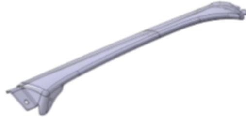
**Figure III-35: Solid model of A-pillar component (~650 mm overall component length).**
