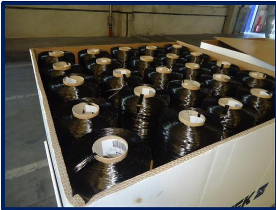
**Figure IV-15: 1500 meter spools of lignin / PAN carbon fiber ready for shipment.**
