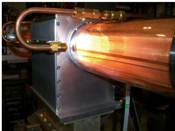
**Figure IV-7: Improved microwave energy and enhanced plasma hardware. This approach, here demonstrated with a single unit, should allow improved energy deposition control for industrial scale-up.**
