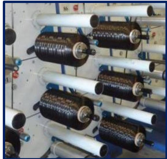
Figure IV-14: Spools of lignin / PAN carbon fiber.
