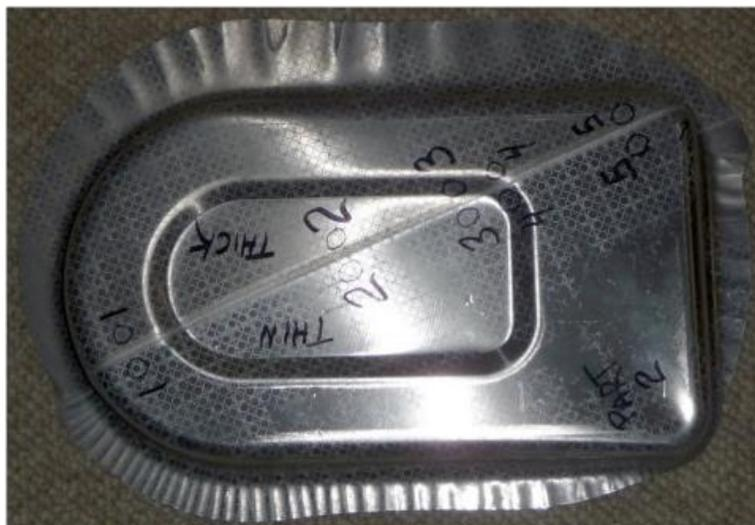
Figure III-80: An as-stamped AA5182 welded blank with 2.0- to 1.2-mm dissimilar thickness sheets.
