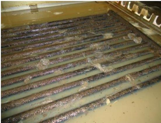
Figure IV-12: Heater coil in pre-stretching bath saturated with non-soluble residue during commercial spinning trial.
