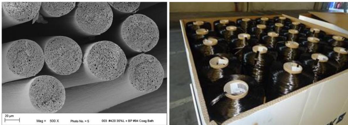
**Figure I-1: 35% lignin/PAN precursor fiber Scanning Electron Microscope image showing uniform micro-porosity and 1500 meter spools of lignin/PAN carbon fiber ready for shipment.**
