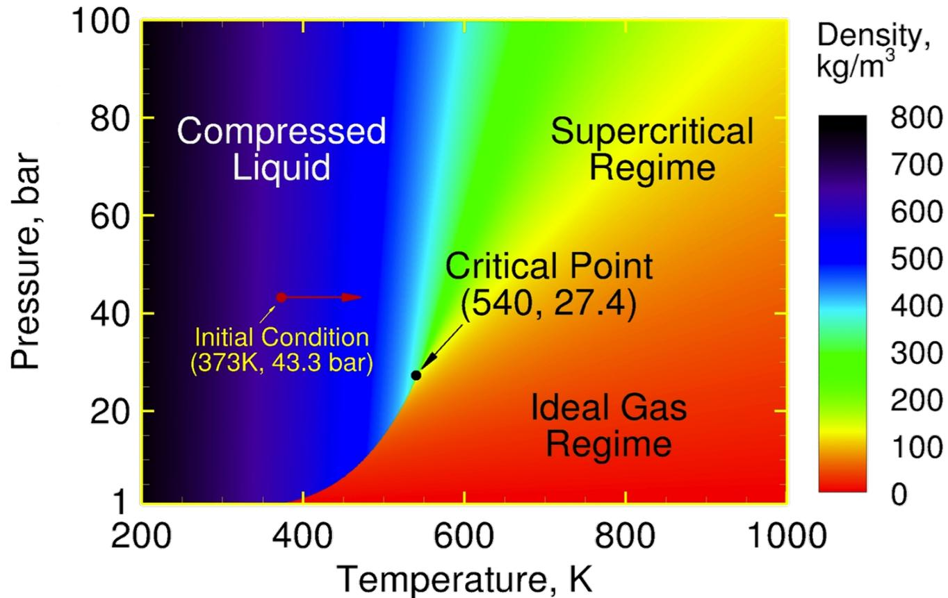
**n-Heptane is being injected as a compressed liquid at supercritical pressure**
