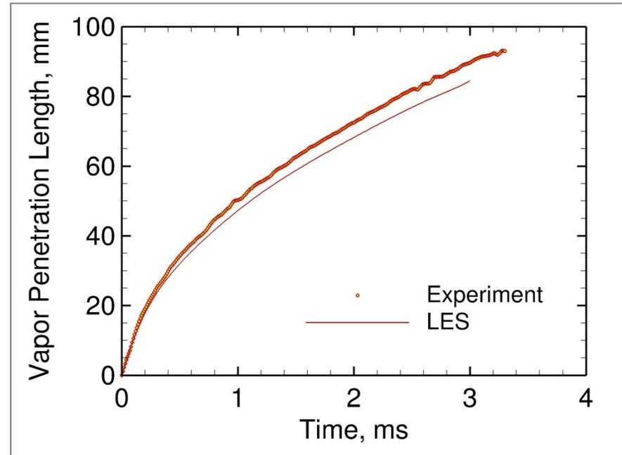
**Mixture fraction thresholds of 0.86 and 0.05, respectively, produce reasonable agreement without the use of tuning constants**
