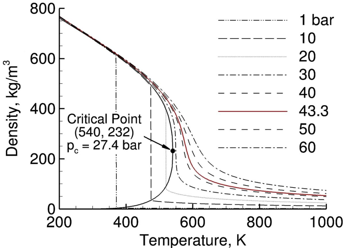
**n-Heptane is being injected as a compressed liquid at supercritical pressure**
