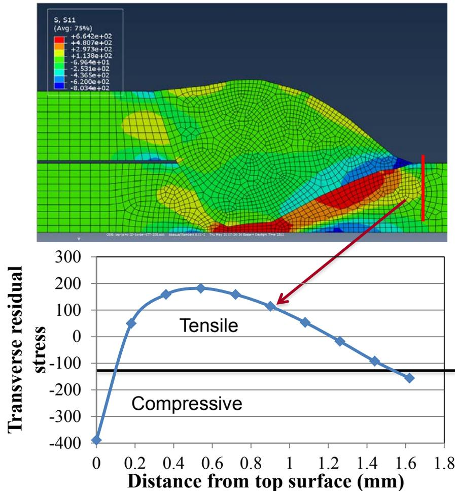
Compressive transverse weld residual stress near weld toe
