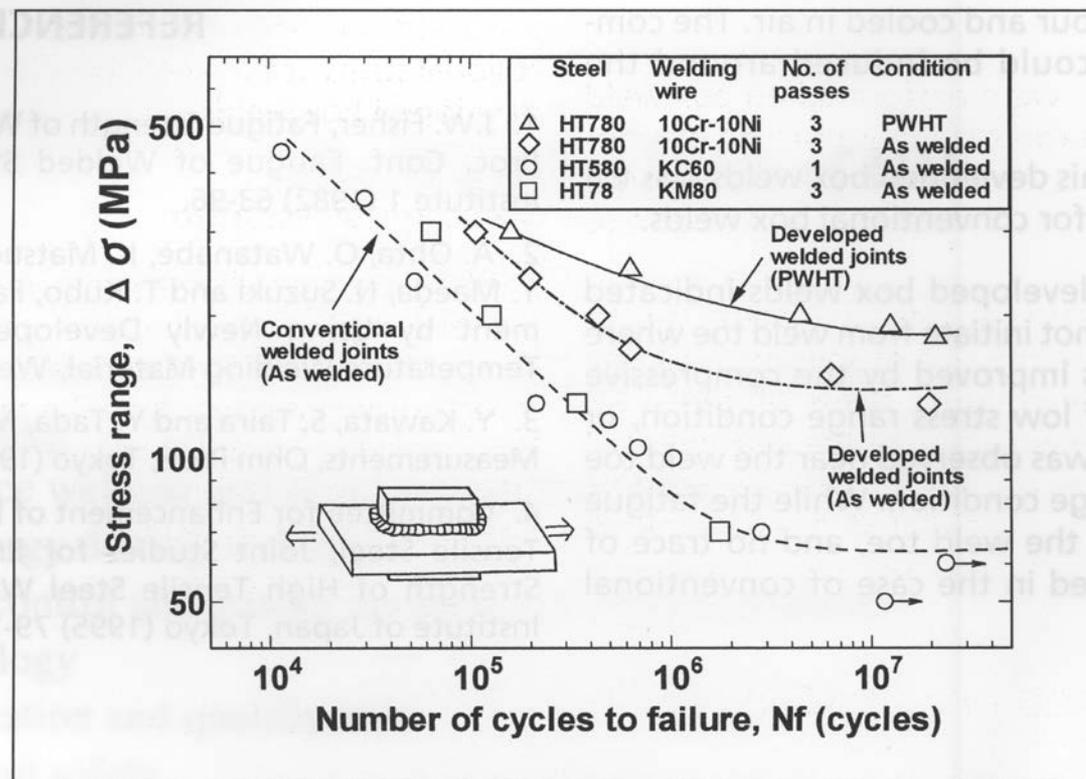
Fig. 6. S-N diagram of box welded joints.
