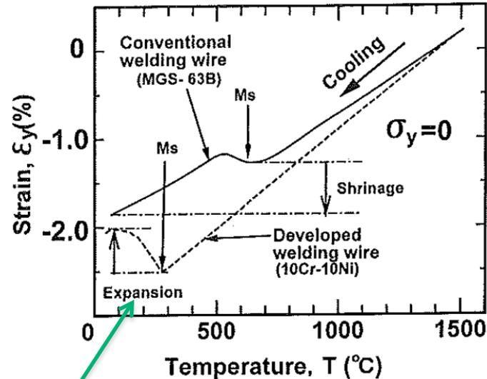
LTT filler metal: phase transformation accrues at low temperature (about 300 °C in this material)
