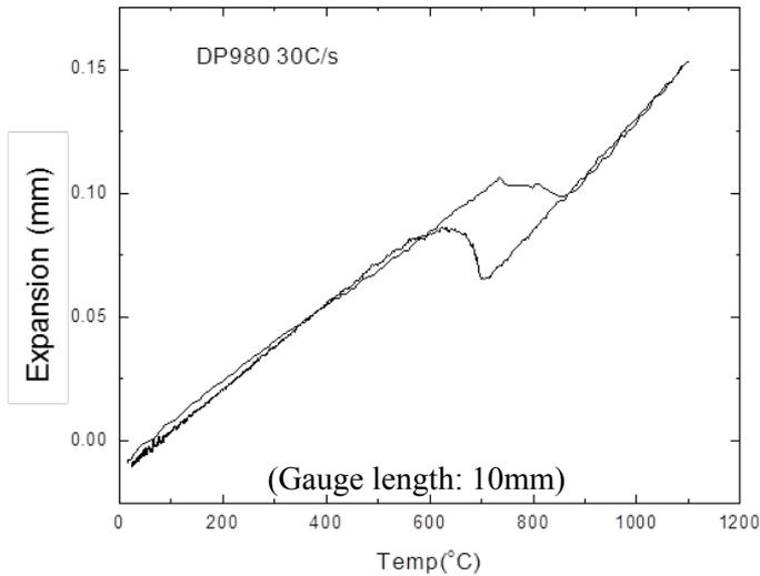
Base metal: phase transformation accrues at high temperature\* (about 700 °C in this material)
