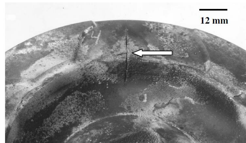
Heavily oxidized MAS piston with crack
