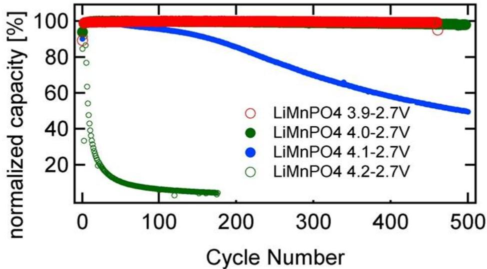
At high voltages with LMP, capacity fades rapidly using current polymer electrolytes
