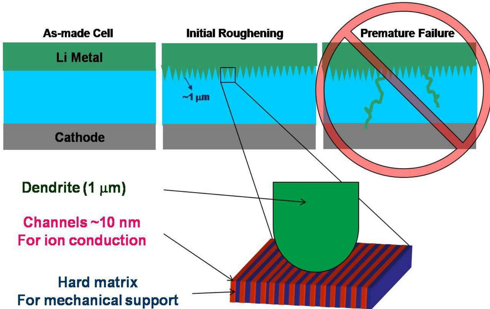
Schematic of the mechanism of dendrite growth inhibition by Seeo's solid polymer electrolyte
