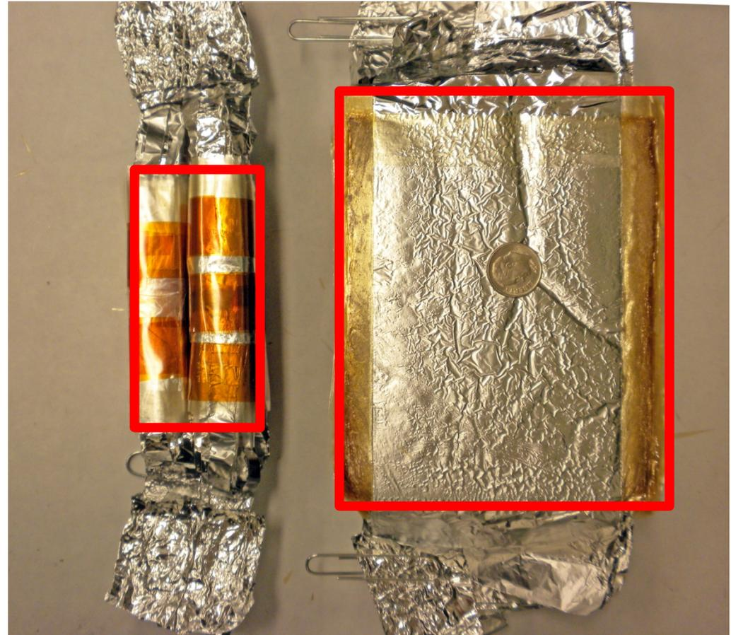
~1  $\mu\text{F}$  rolled pressed capacitor
