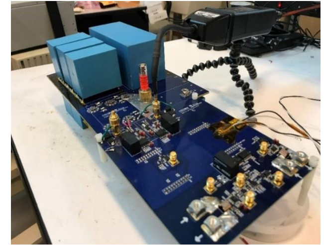
Fig. 12 Current sensing evaluation hardware testbed
