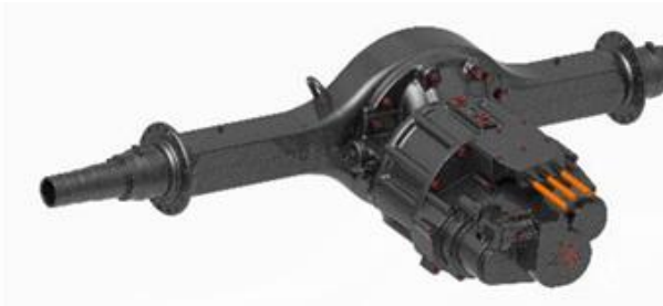
Fig. 12 Meritor eAxle specification
