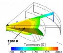
(UW) Model predictions show efficiency is improved by combustion design to reduce heat transfer
